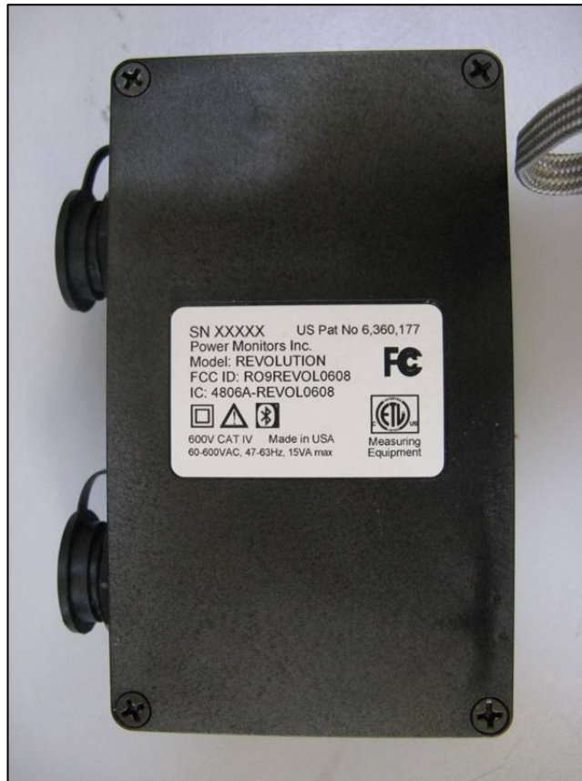
Photograph 1: ID Label and Location
