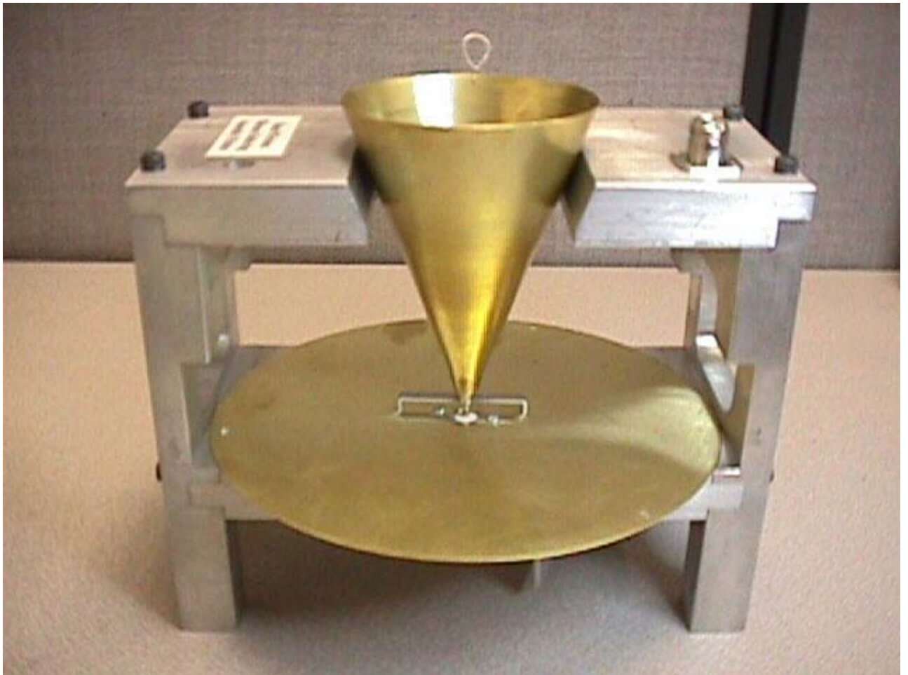
Discone Antenna, internal view:
