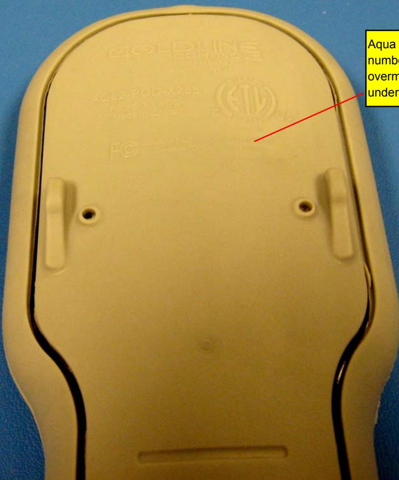
Aqua Pod label location. The FCC ID number is molded into the plastic overmold on the bottom of the unit underneath the LCD.
