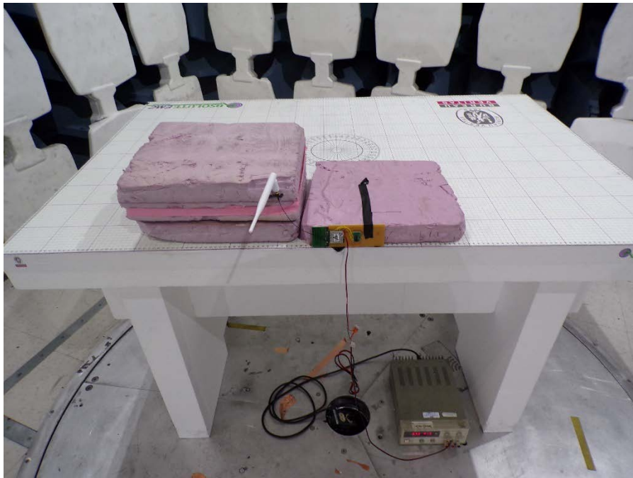
Module: Y-Axis External Antenna: Horizontal (Worst Case Orientation)
