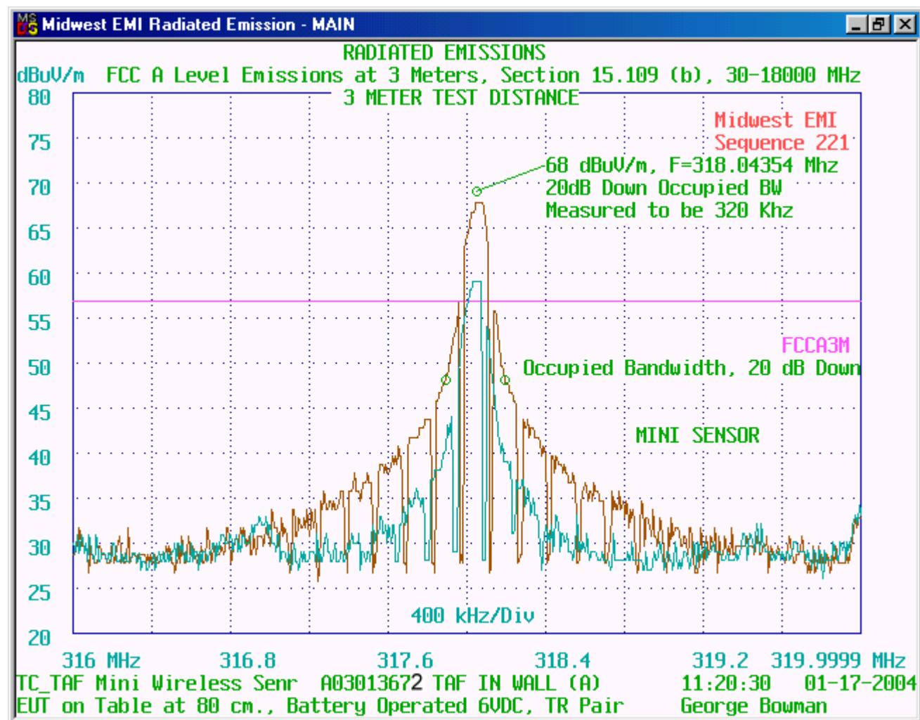
The 20 dB down occupied bandwidth is 328 KHz and measured as a percent is .103% meeting the FCC requirement of .25% (15.231 (c)). [This and any other data taken on the 3 meter site used a Tek 2712 with EMC option SN B022981 calibrated on 27 Aug 03. The antenna used is a linearly polarized Antenna Research LPB 2520 SN 1151 calibrated on 27 Oct 03. A 20 dB calibrated
