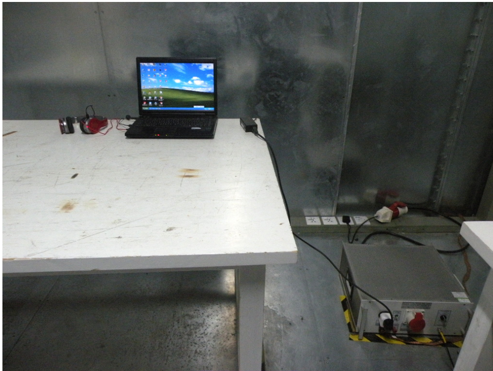
Radiated Emission Test Setup in Chamber
