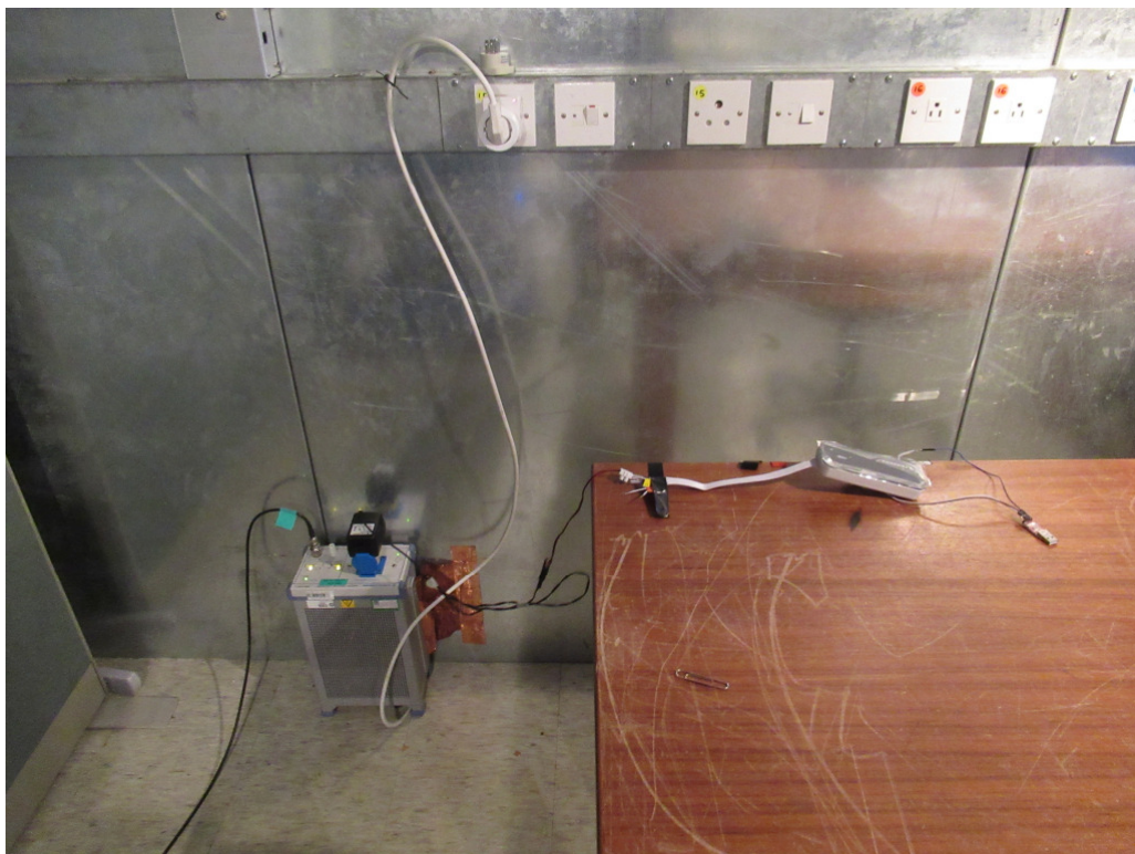
Set-up for AC Conducted Emission (worst case)
