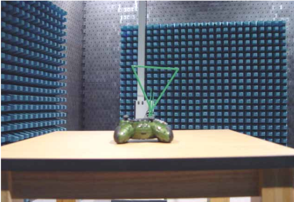
Radiation Emission Test setup
