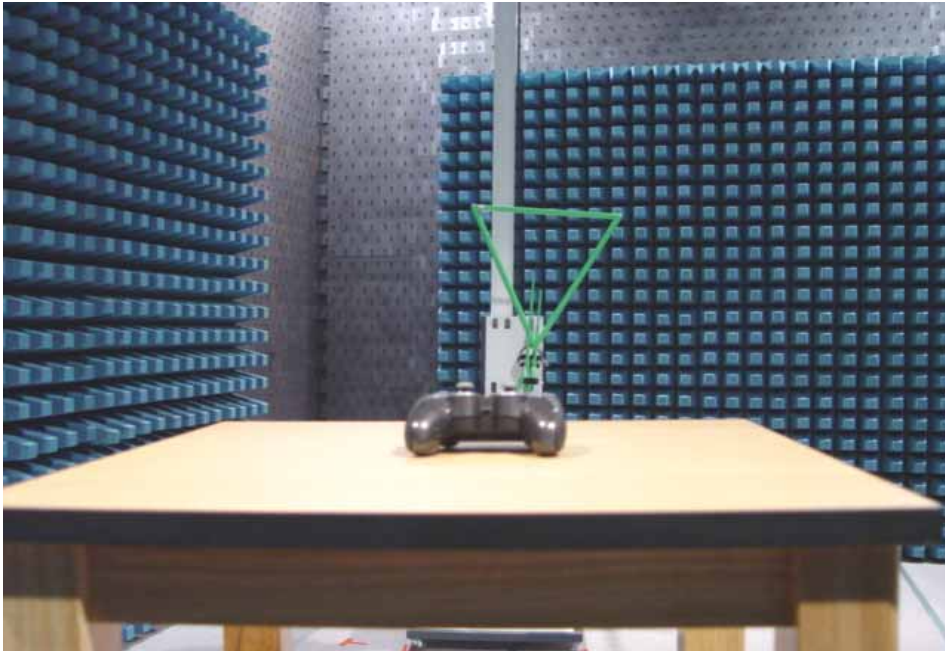
Radiation Emission Test setup
