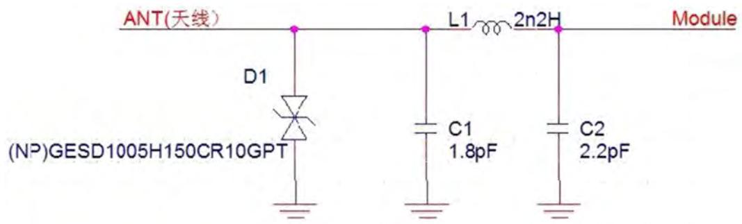
9.1.1 Above the dotted box part of the antenna matching is needed, the actual antenna matching electronic parameters shall prevail.
