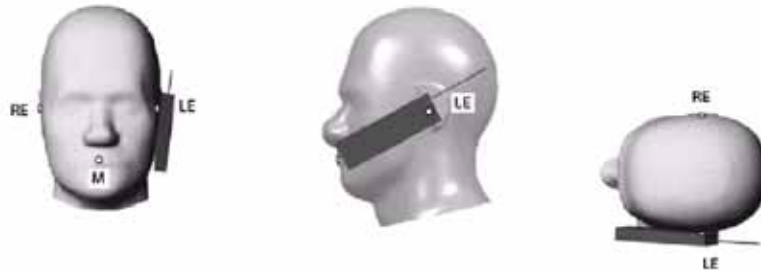
Figure 5.4 Front, Side and Top View of Cheek/Touch Position
