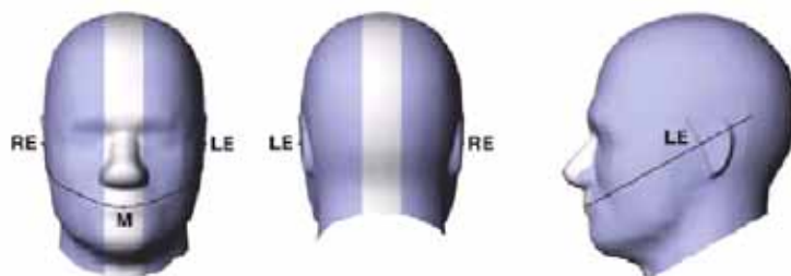
Figure 5.1 Front, back and side view of SAM Twin Phantom
