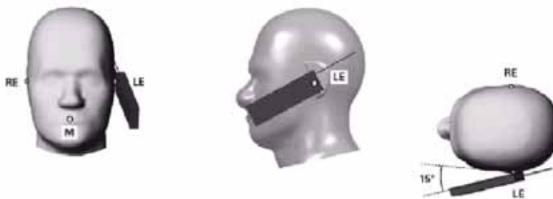
Figure 5.6 Front, Side and Top View of Ear/15° Tilt Position
