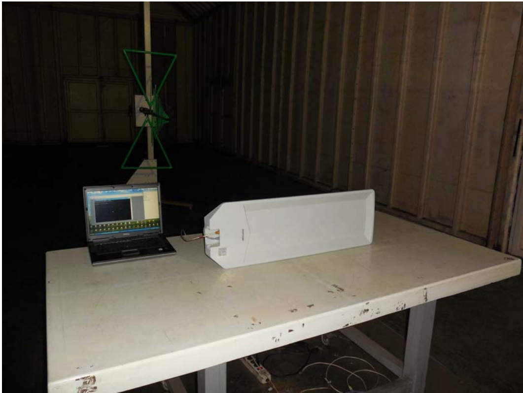
Front View of Radiated Test
