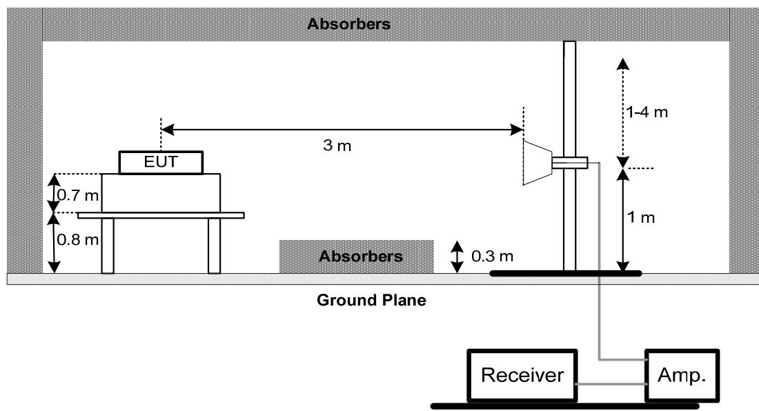
(C) For radiated emissions below 30MHz
