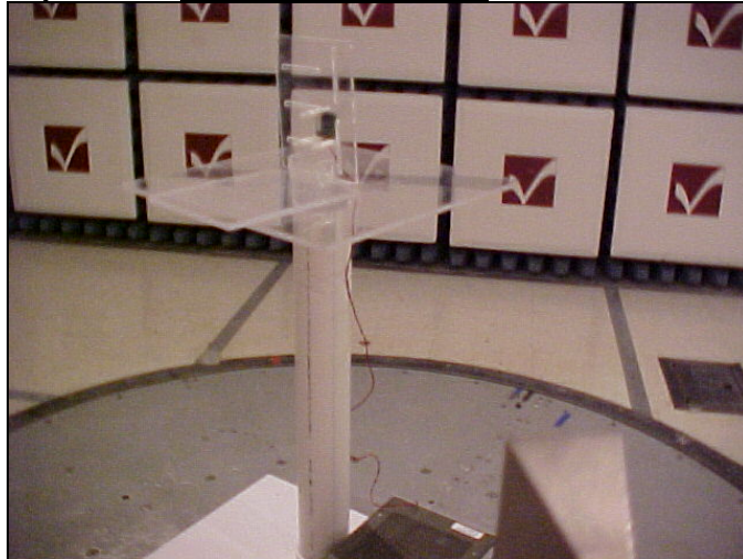
Setup for the Radiated Emissions Test, Side Position
