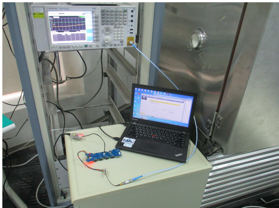
Photograph 5: Set-up for Conducted testing
