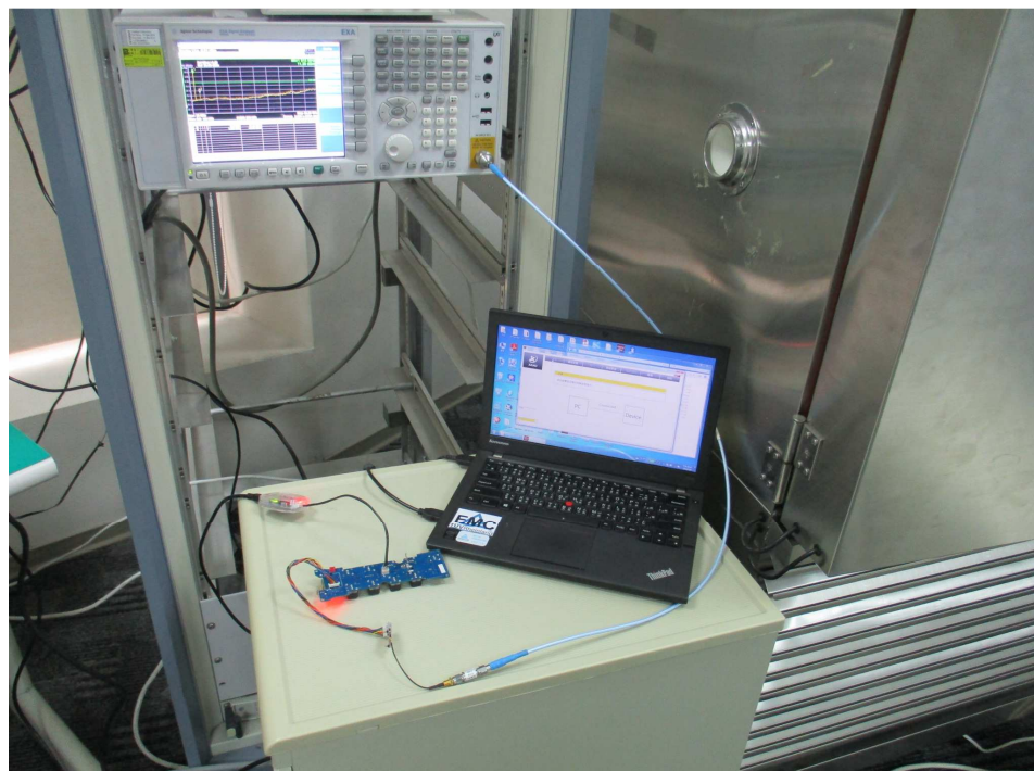
Photograph 5: Set-up for Conducted testing
