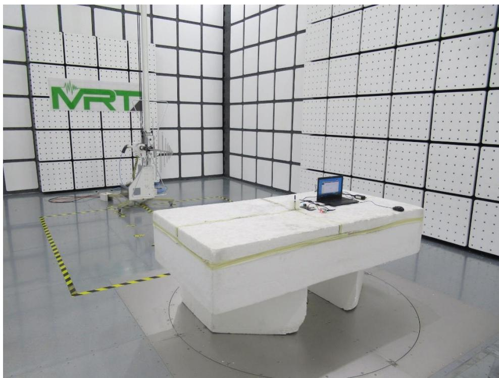
**Transmit - 2.4GHz with Dipole Antenna****Description:** Radiated Emission Test Setup for above 1GHz
