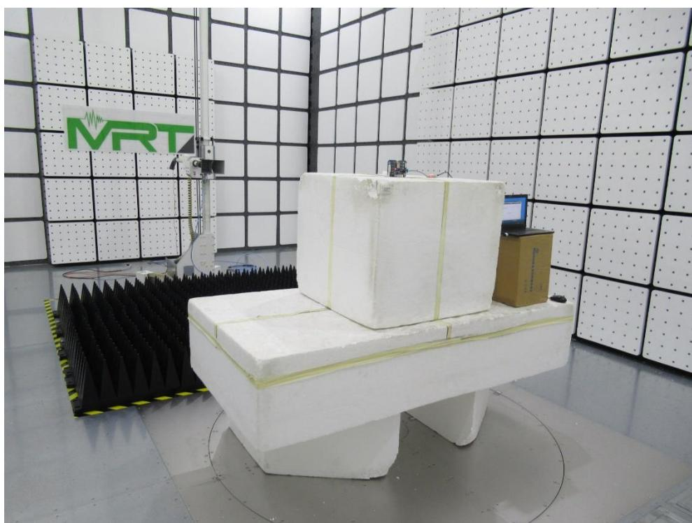
**Description: Conducted Emission Test Setup**
