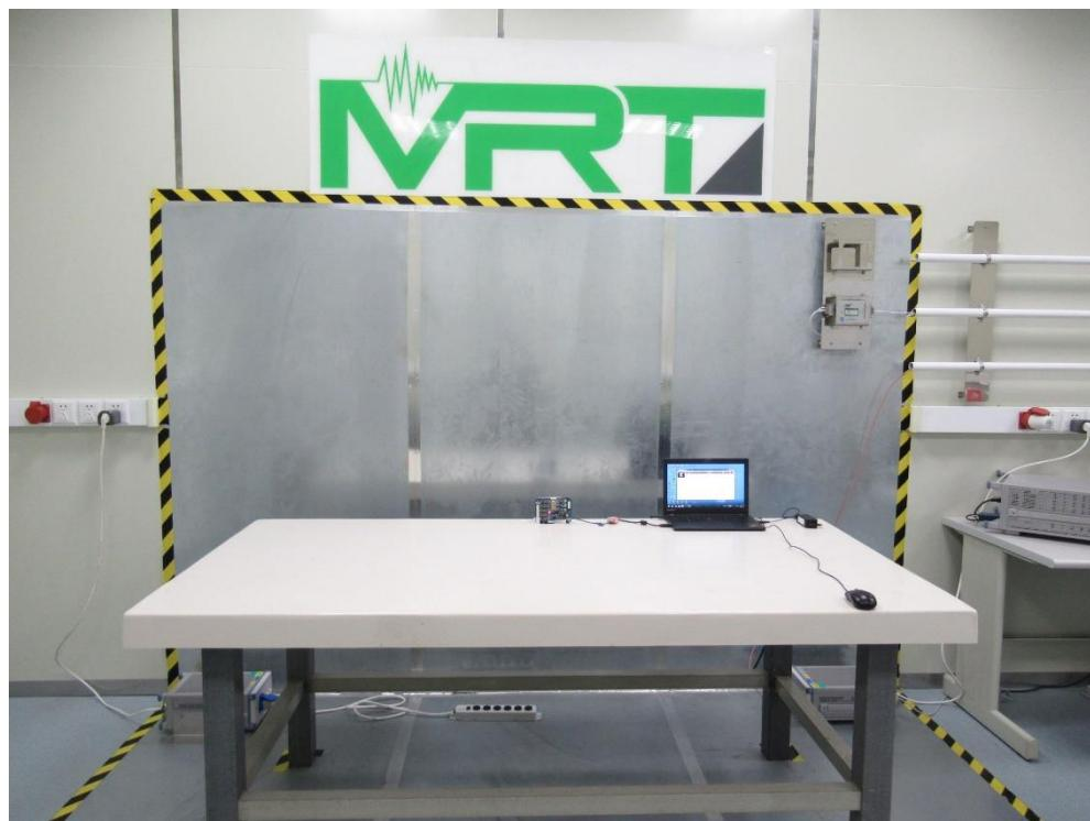
**Transmit – 2.4GHz with PCB Antenna****Description: Back View of Conducted Emission Test Setup**
