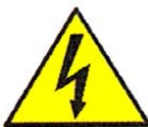
All parts making up the equipment have danger identification tags (with a yellow background) to highlight the parts dangerous for the operator that has access to the system
