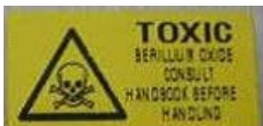
This warning label is used for components containing Beryllium Oxide.
