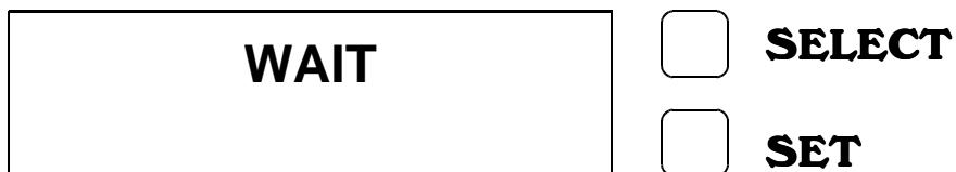
After few seconds the green PLL LOCK led will light and the Display will show an increasing bar; after a further 5 seconds the green ON AIR LED will light and the unit will start increasing power.
