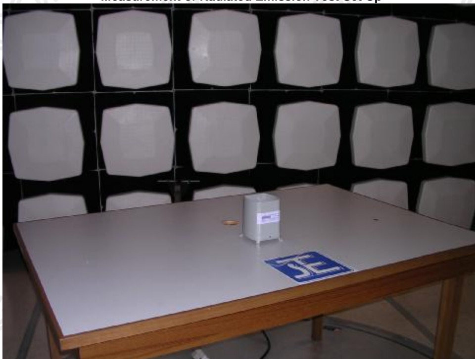
Measurement of Radiated Emission Test Set Up
