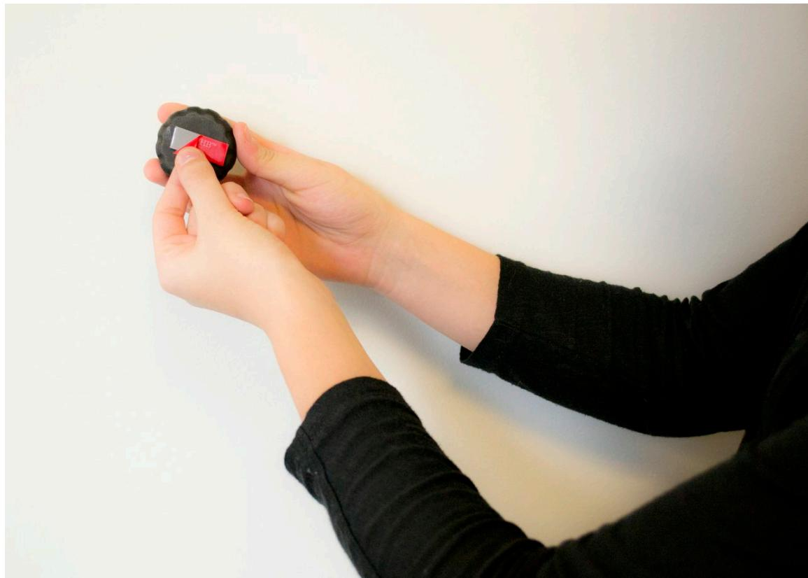
7. To remove the sensor from a wall or fixture, twist the bottom section of the sensor case in either a clockwise or counter clockwise manner until the adhesive separates from the case leaving it exposed on the wall or fixture. Remove the adhesive left behind by scraping a corner with your fingertip and peeling and rolling into a ball until it's fully removed.
