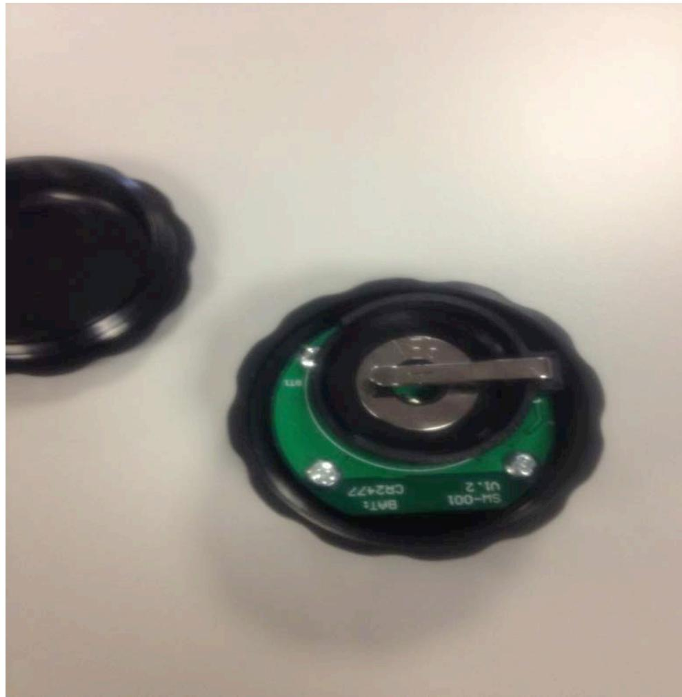
3. Place the provided CR2477 3V battery in the battery holder by positioning the positive (+) marked face of the battery in the upright position. Slide the battery into the holder at an angle pushing the battery towards the back of the holder until it snaps into place and sits flush.
