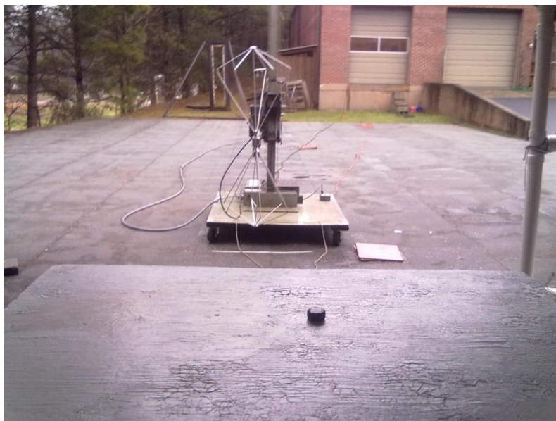
Photo 3 – Test Configuration of the EUT Above 30 MHz Testing
