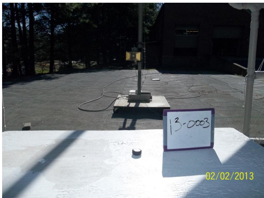
Photo 3 – Test Configuration of the EUT Above 1 GHz Testing
