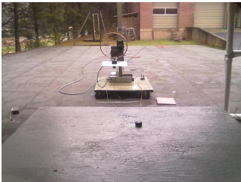
Photo 2 – Test Configuration of EUT Below 30 MHz Testing
