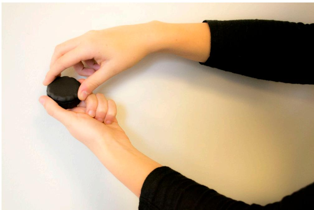
5. Once the battery is properly installed, the Swirl Sensor will automatically start broadcasting and advertising its presence. The
