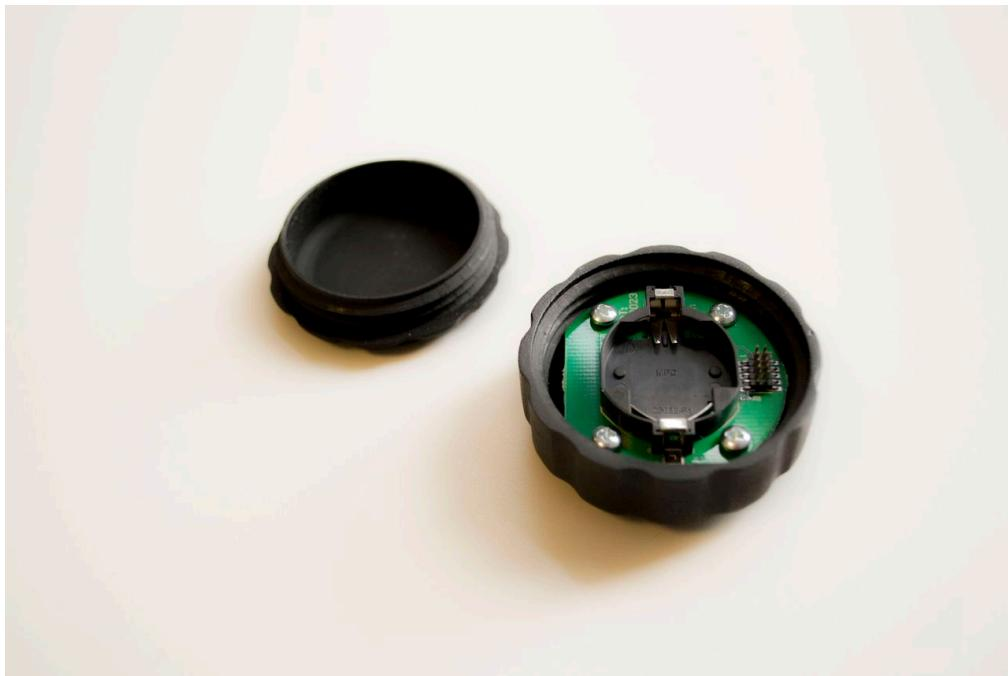
3. Place the provided CR2032 3V battery in the battery holder by positioning the positive (+) marked face of the battery in the upright position. Slide the battery into the holder at an angle pushing the battery beyond the two protruded plastic guards and against the rounded metal guards. Once guards are cleared, slightly push the battery down allowing it to snap firmly into place.
