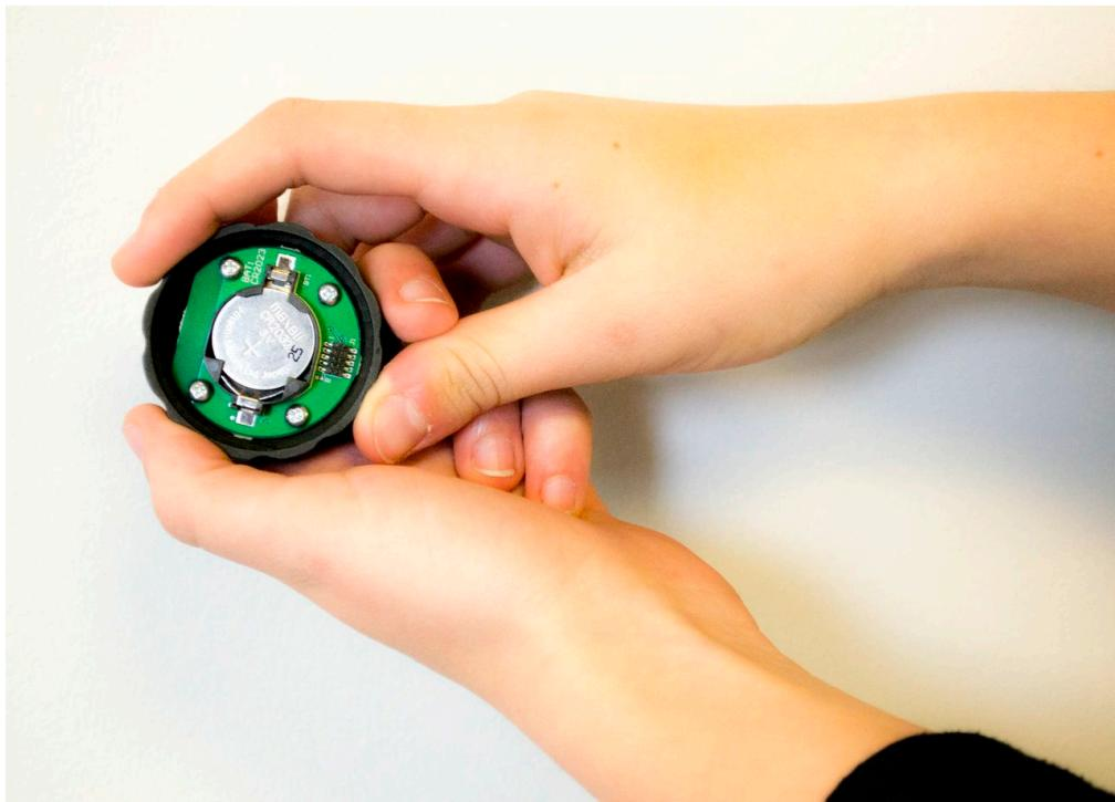
4. Re-assemble the top and bottom case section by screwing together until snug. Do not over tighten
