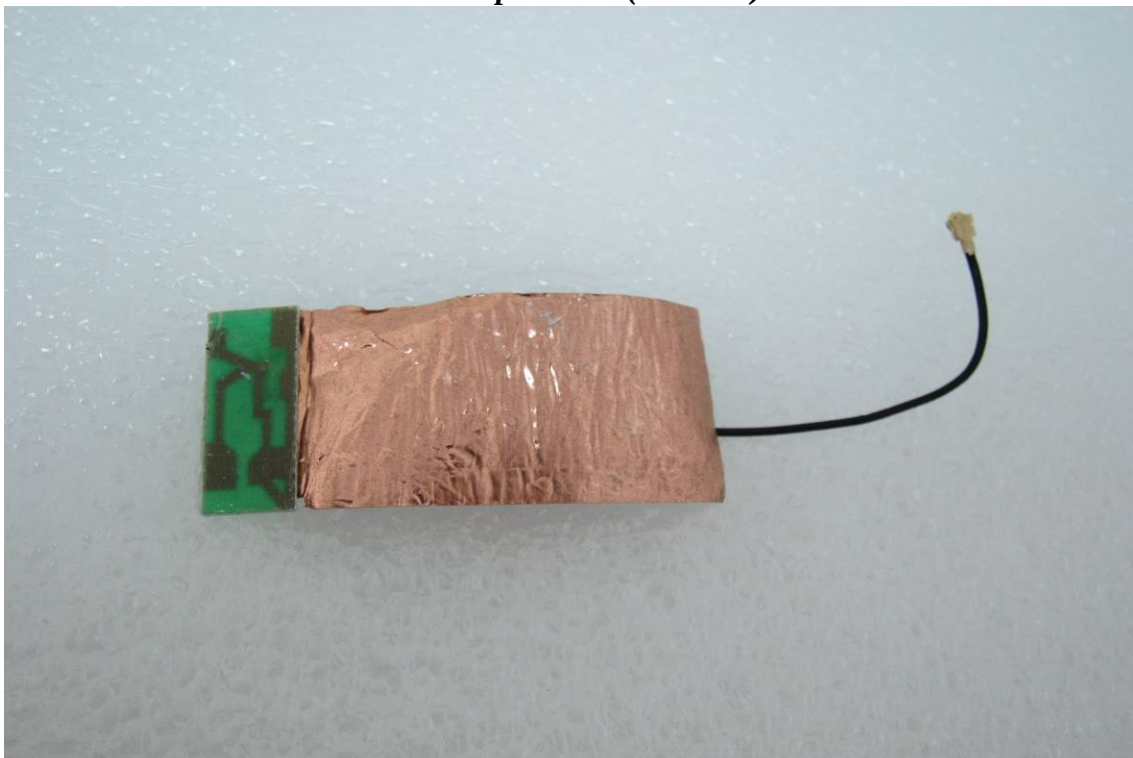
Internal photo – 6 (Antenna)
