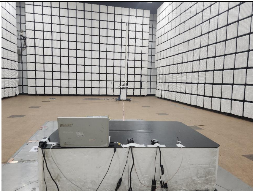
[Rear view of Radiated Emission (30 MHz ~ 1 000 MHz)]
