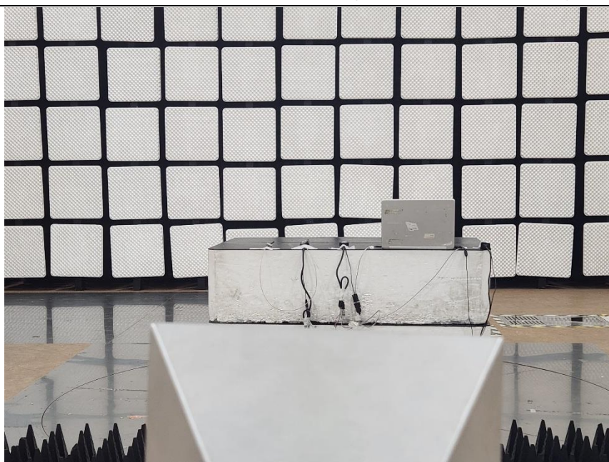
[Rear view of Radiated Emission (1 000 MHz ~ 30 000 MHz)]
