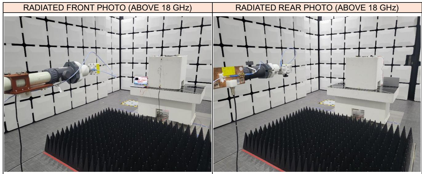
**RADIATED RF MEASUREMENT SETUP FOR PORTABLE CONFIGURATION**
