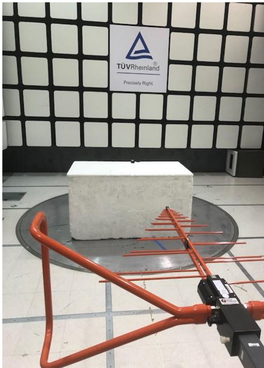
Figure 5 - Radiated Emissions Test Setup 30 - 1000 MHz – Front
