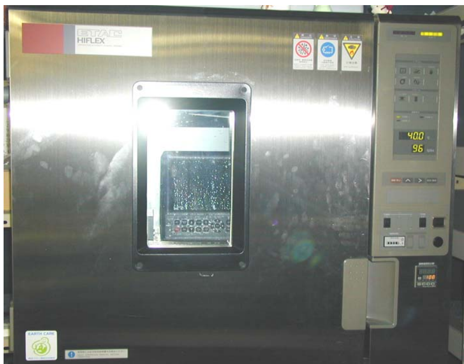
Photo 12: View of EUT in Model FX206C Constant Temperature Test Chamber 24th June, 2005 at 16:49 (Chamber set to 40 \pm 2^\circ \text{C} and 90 to 95% RH)
