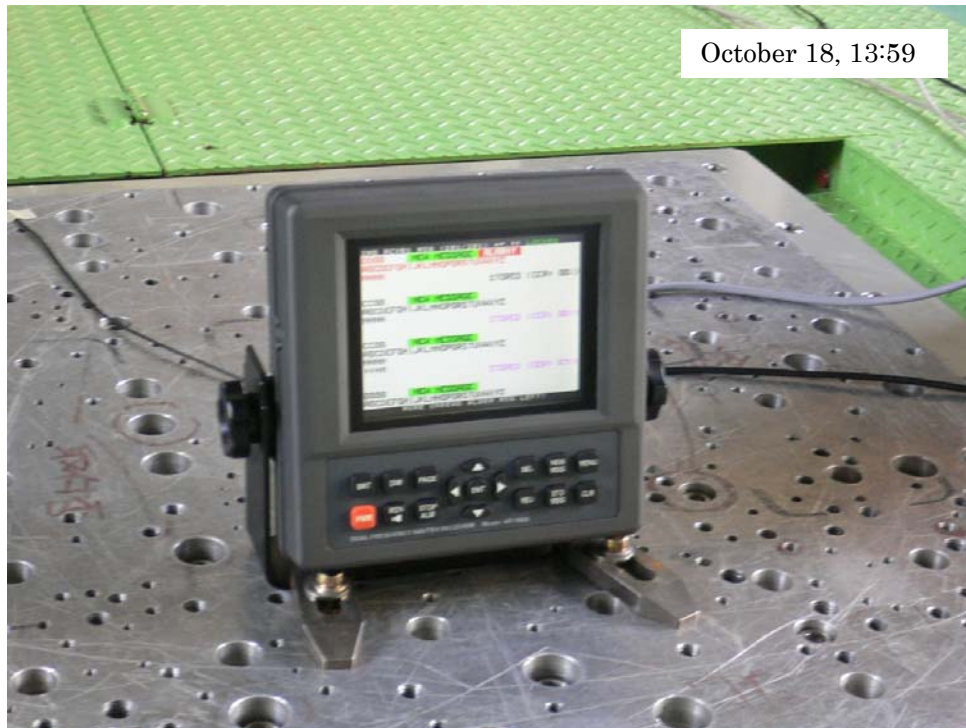
Photo-9: Checking EUT's Sensitivity before Starting 2-Hour X-Axis Endurance Test at Resonance – 2/2
