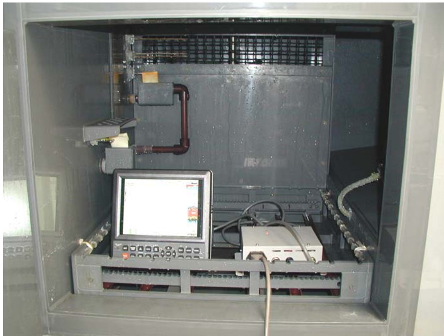
Photo 10: View of EUT Just before Start of 3rd Saltwater Mist Spray Test 24th June, 2005 at 13:35
