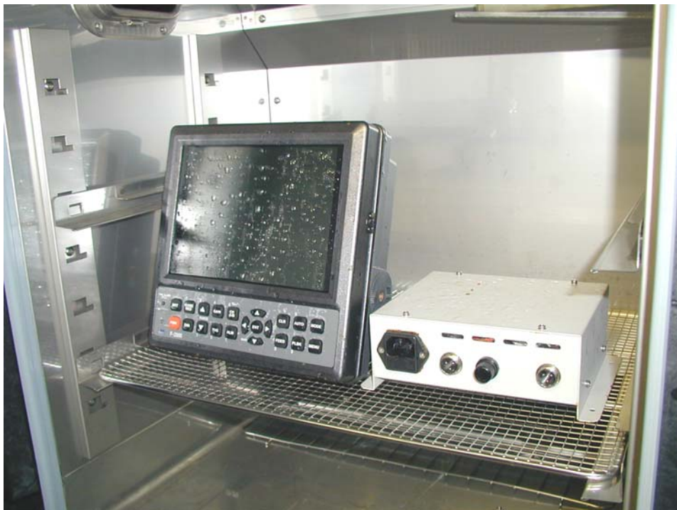
Photo 14: View (2) Of EUT Just after Completion of 4th Saltwater Mist Spray Test 1st July, 2005 at 15:42
