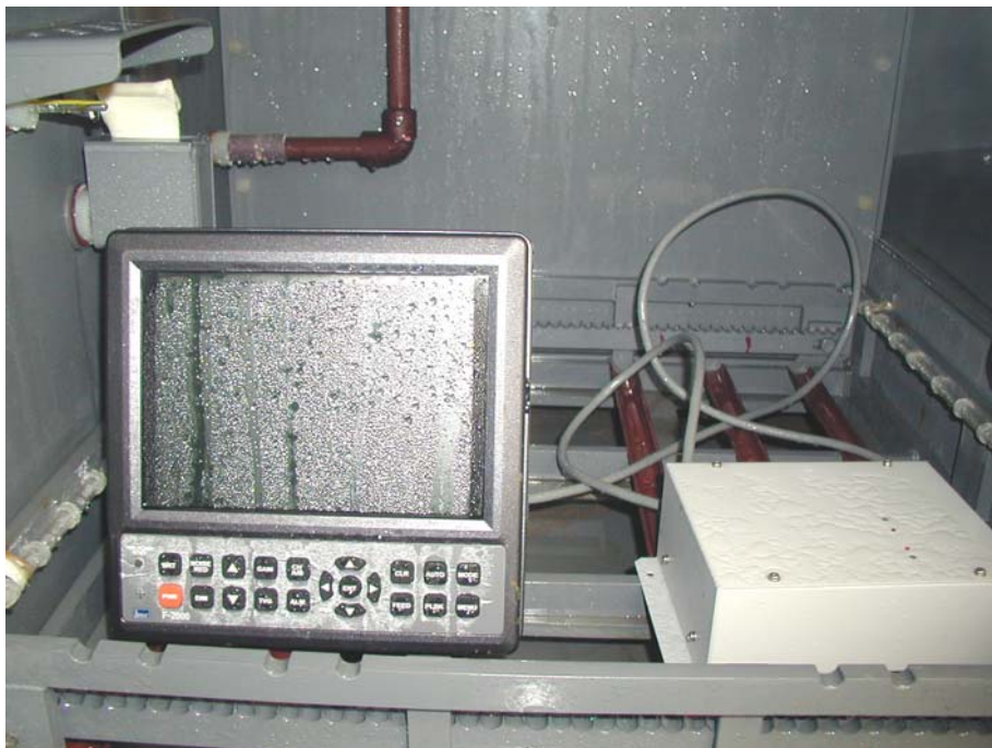
Photo 8: View of EUT Just after Completion of 2nd Saltwater Mist Spray Test 17th June, 2005 at 15:41
