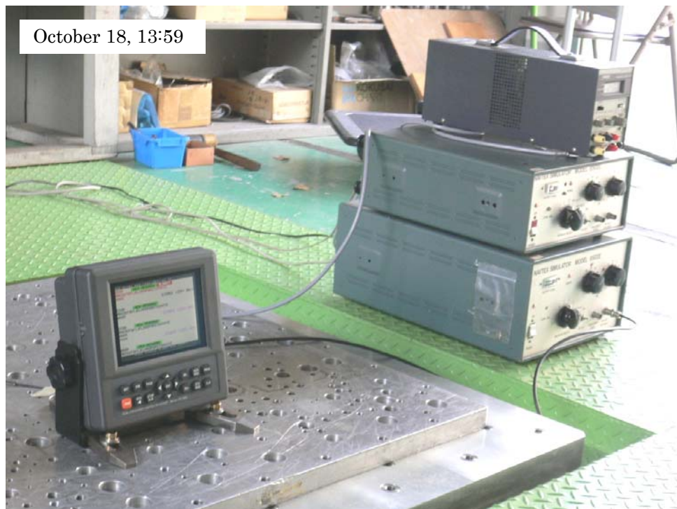
Photo-8: Checking EUT's Sensitivity before Starting 2-Hour X-Axis Endurance Test at Resonance – 1/2
