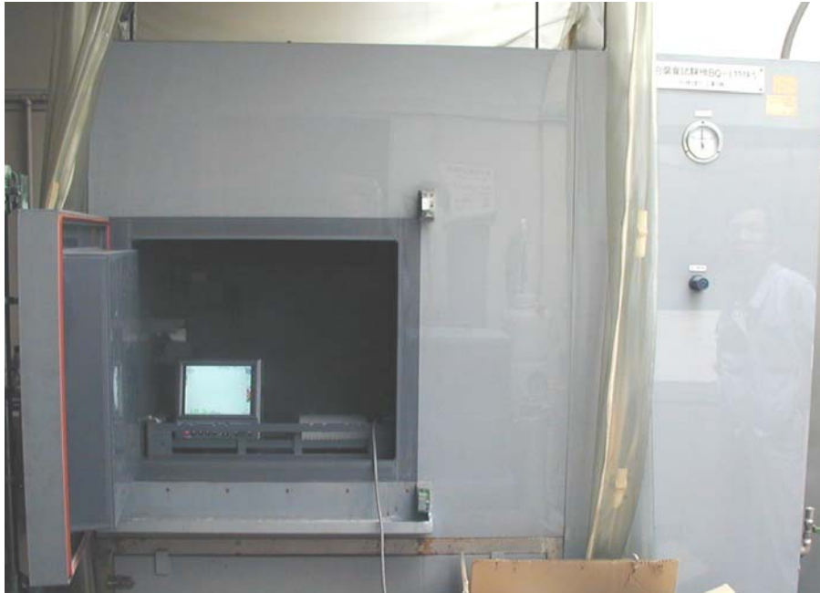
Photo 7: View of EUT Just before Start of 2nd Saltwater Mist Spray Test 17th June, 2005 at 13:39
