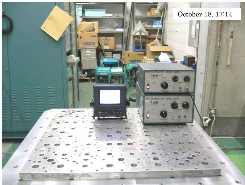
Photo-11: Checking EUT's Sensitivity before Starting Z-Axis Test
