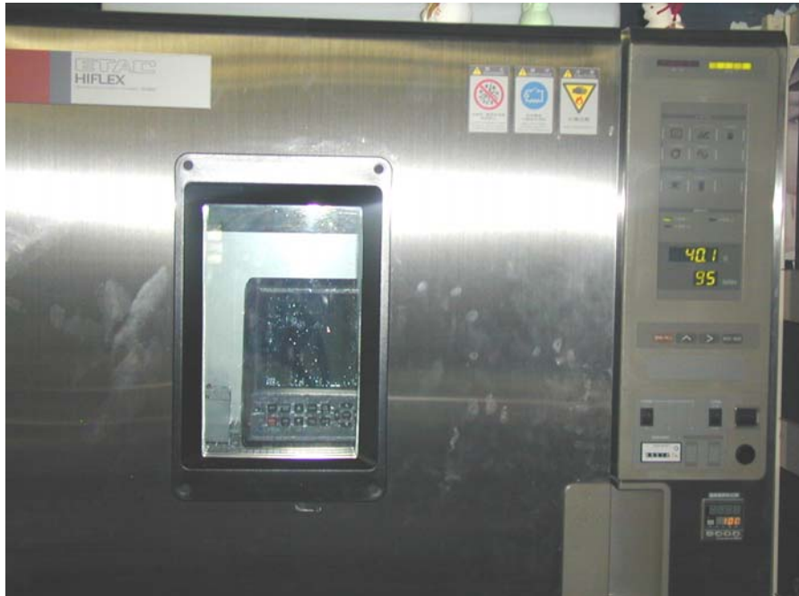
Photo 9: View of EUT in Model FX206C Constant Temperature Test Chamber 17th June, 2005 at 17:06 (Chamber set to 40 \pm 2^\circ \text{C} and 90 to 95% RH)
