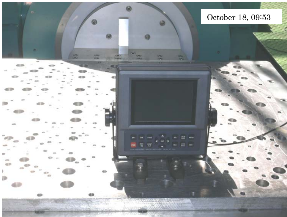
Photo-3: EUT Placed on Slip Table before Starting Y-Axis Test – 1/2
