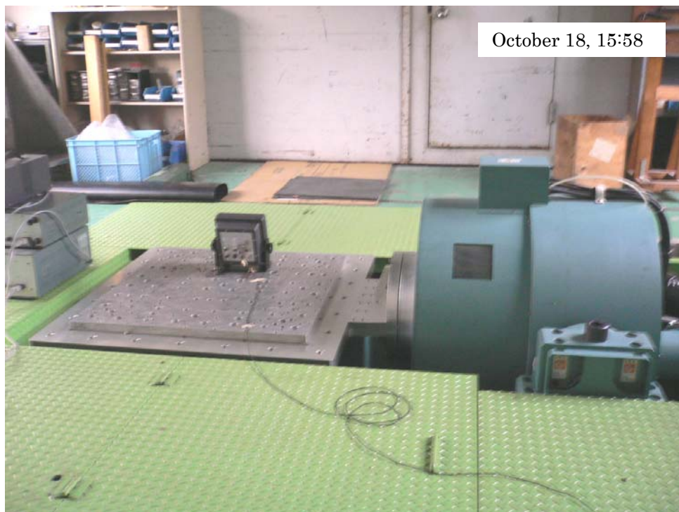
Photo-10: 2-Hour X-Axis Endurance Test at Resonance in Progress
