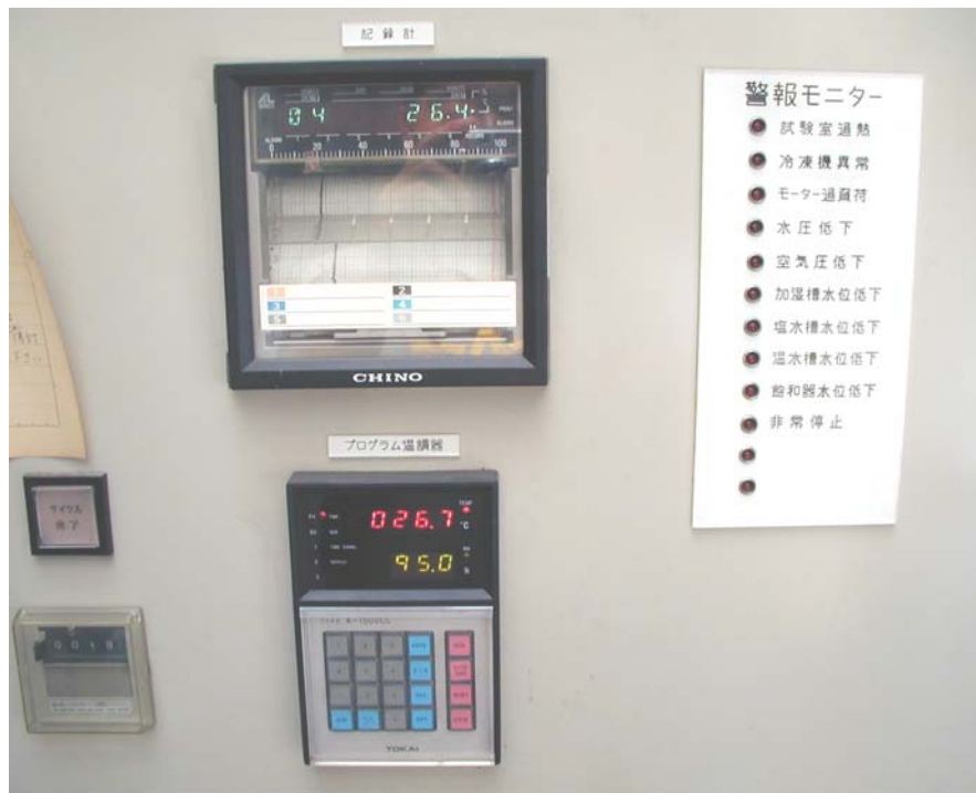
Photo 3: Front View (2) of Model BQ-1 Complex Corrosion Tester (Recorder, Programmable Temp. Controller, Alarm Monitor Lamps)
