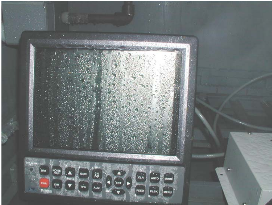
Photo 13: View (1) of EUT Just after Completion of 4th Saltwater Mist Spray Test 1st July, 2005 at 15:42
