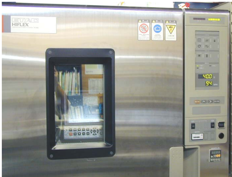
Photo 6: View of EUT in Model FX206C Constant Temperature Test Chamber 10th June, 2005 at 17:57 (Chamber set to 40 \pm 2^{\circ}\text{C} and 90 to 95% RH)
