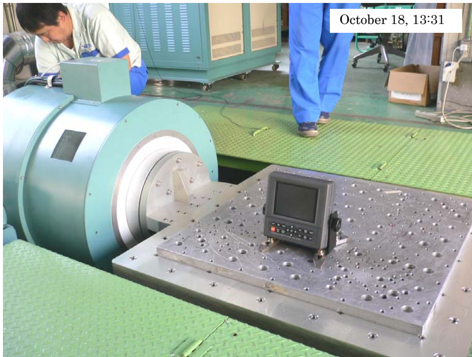
Photo-7: EUT Placed on Slip Table for X-Axis Test
