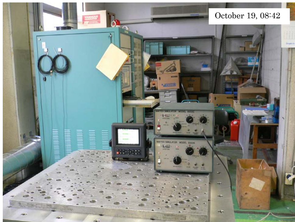
Photo-14: Checking EUT's Sensitivity before Starting 2-Hour Z-Axis Endurance Test at Resonance
