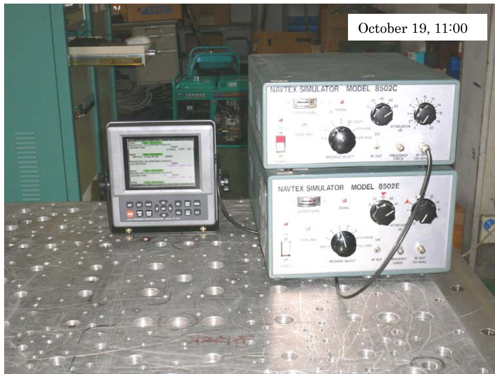
Photo-15: Checking EUT's Sensitivity on Completion of 2-Hour Z-Axis Endurance Test at Resonance
