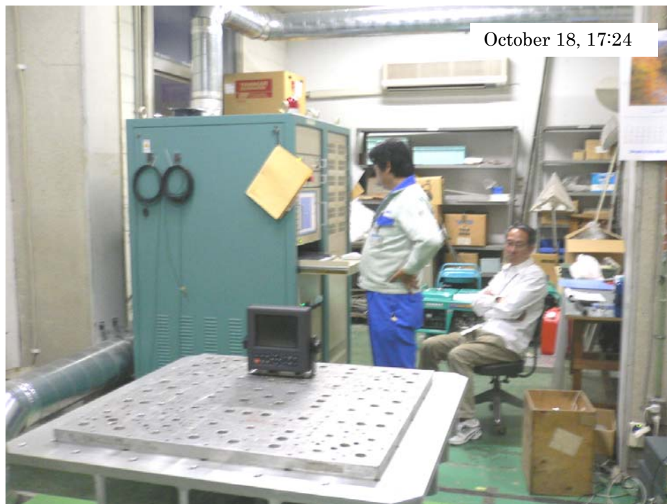
Photo-12: Searching for Resonance in Z-Axis Direction – 1/2
