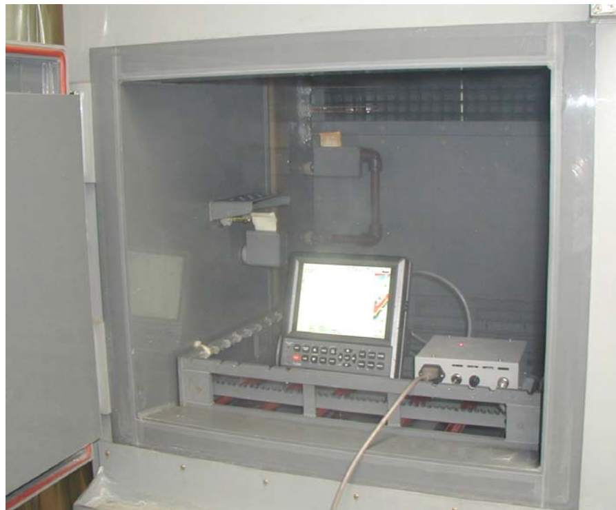
Photo 4: EUT & AC-2000 Placed in Chamber, Just before 1st Saltwater Mist Spray Test 10th June 2005 at 13:37
