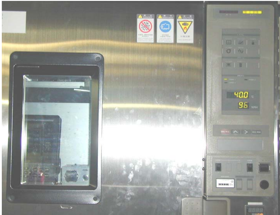
Photo 15: View of EUT in Model FX206C Constant Temperature Test Chamber 1st July, 2005 at 17:30 (Chamber set to 40 \pm 2^{\circ}\text{C} and 90 to 95% RH)
