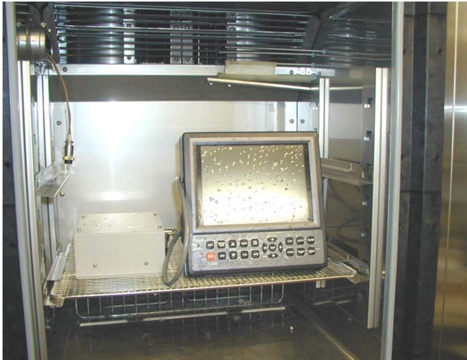
Photo 5: View of EUT Just after Completion of 1st Saltwater Mist Spray Test 10th June, 2005 at 16:52
