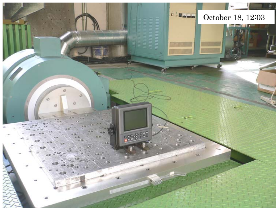
Photo-6: EUT before Completion of 2-Hour Y-Axis Endurance Test at Resonance
