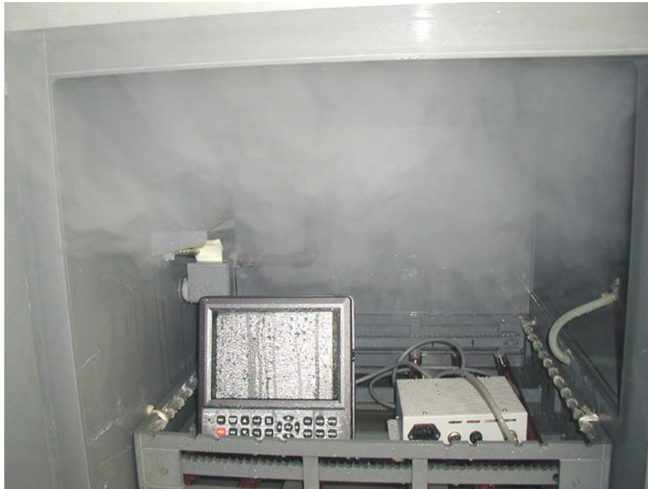
Photo 11: View of EUT Just after Completion of 3rd Saltwater Mist Spray Test 24th June, 2005 at 15:38
