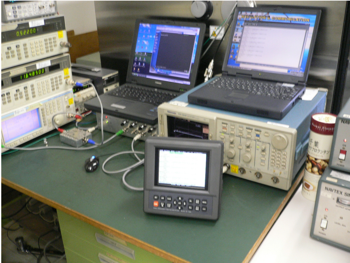
Photo-15: Test System for Testing EUT ( ANT-2000M ) at ( -25^{\circ}\text{C} ) November 23, 2007 at TOKIMEC's Environmental Test Laboratory
