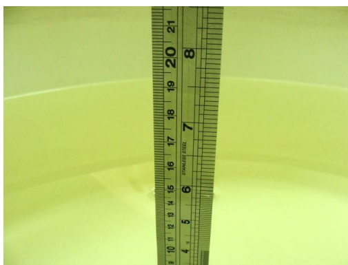
Fig 6.1 Photo of Liquid Height for Body SAR
