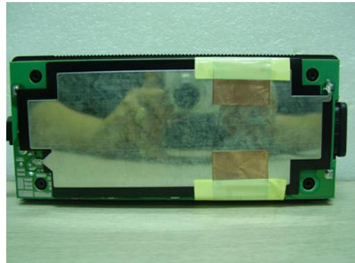
Copper foil tapes are applied to front panel and Adaptor.
