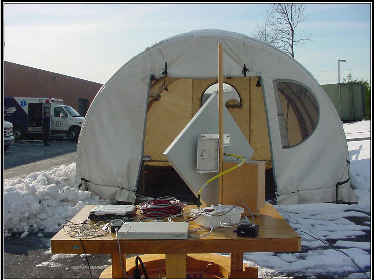
PHOTOGRAPH 2: RADIATED EMISSIONS FRONT VIEW
