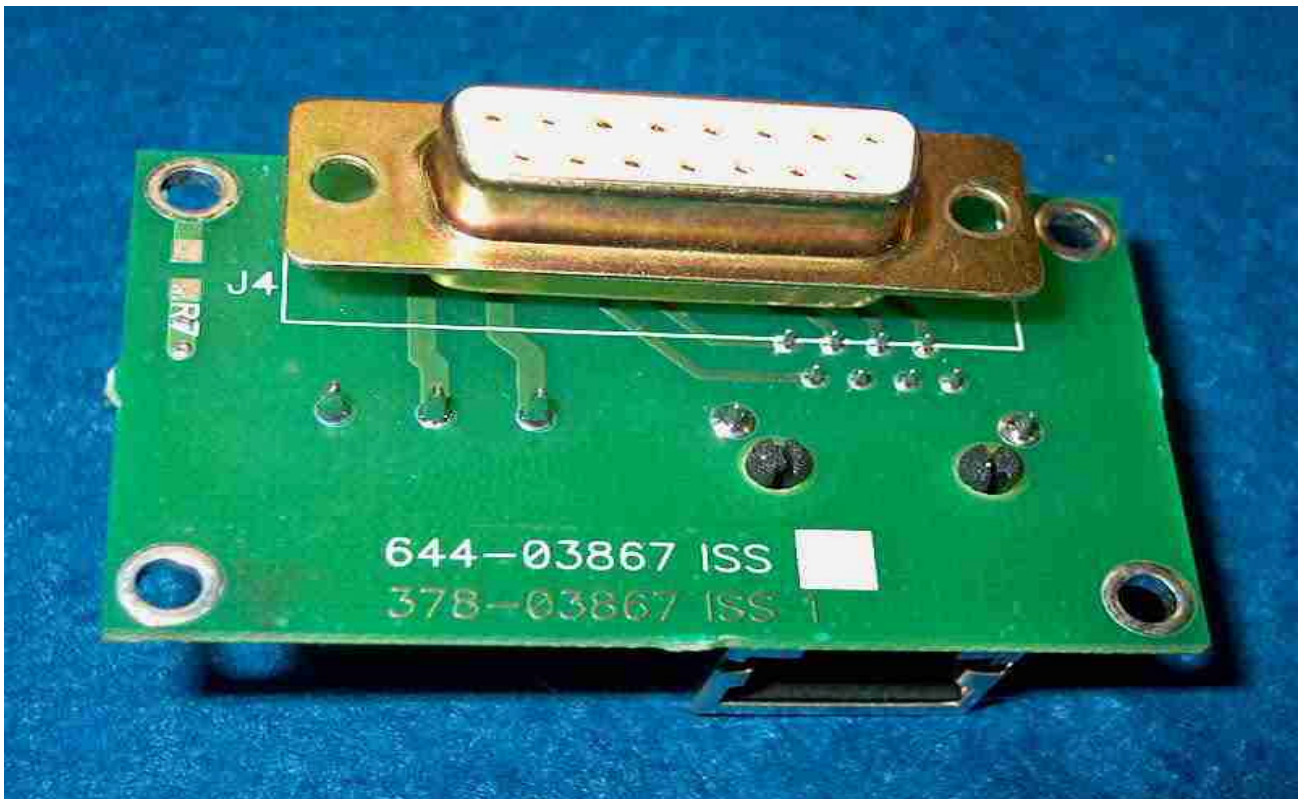
External Cable Interface PCB Top & Bottom
