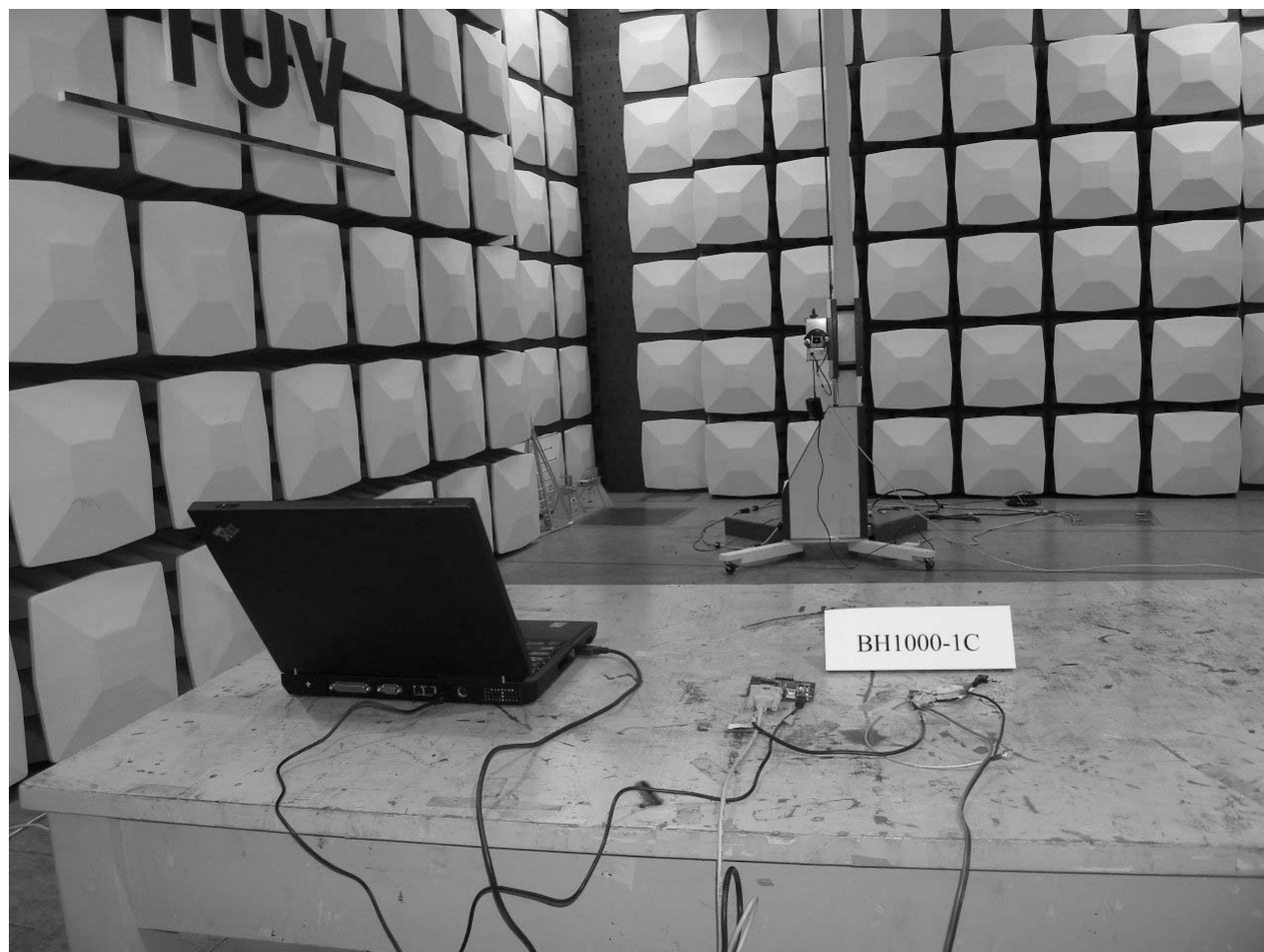
Photograph 1: Set-up for Radiation Measurement below 1GHz
