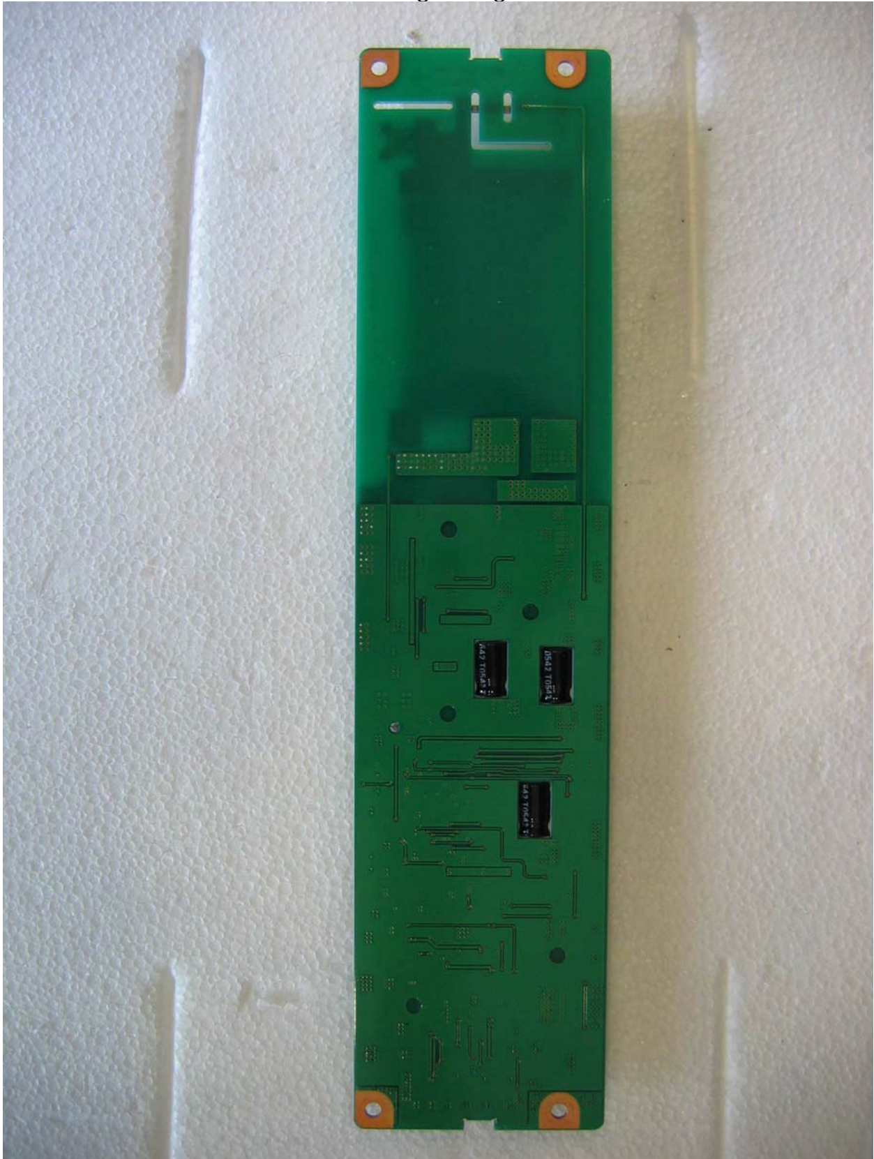
Bottom of high voltage board
