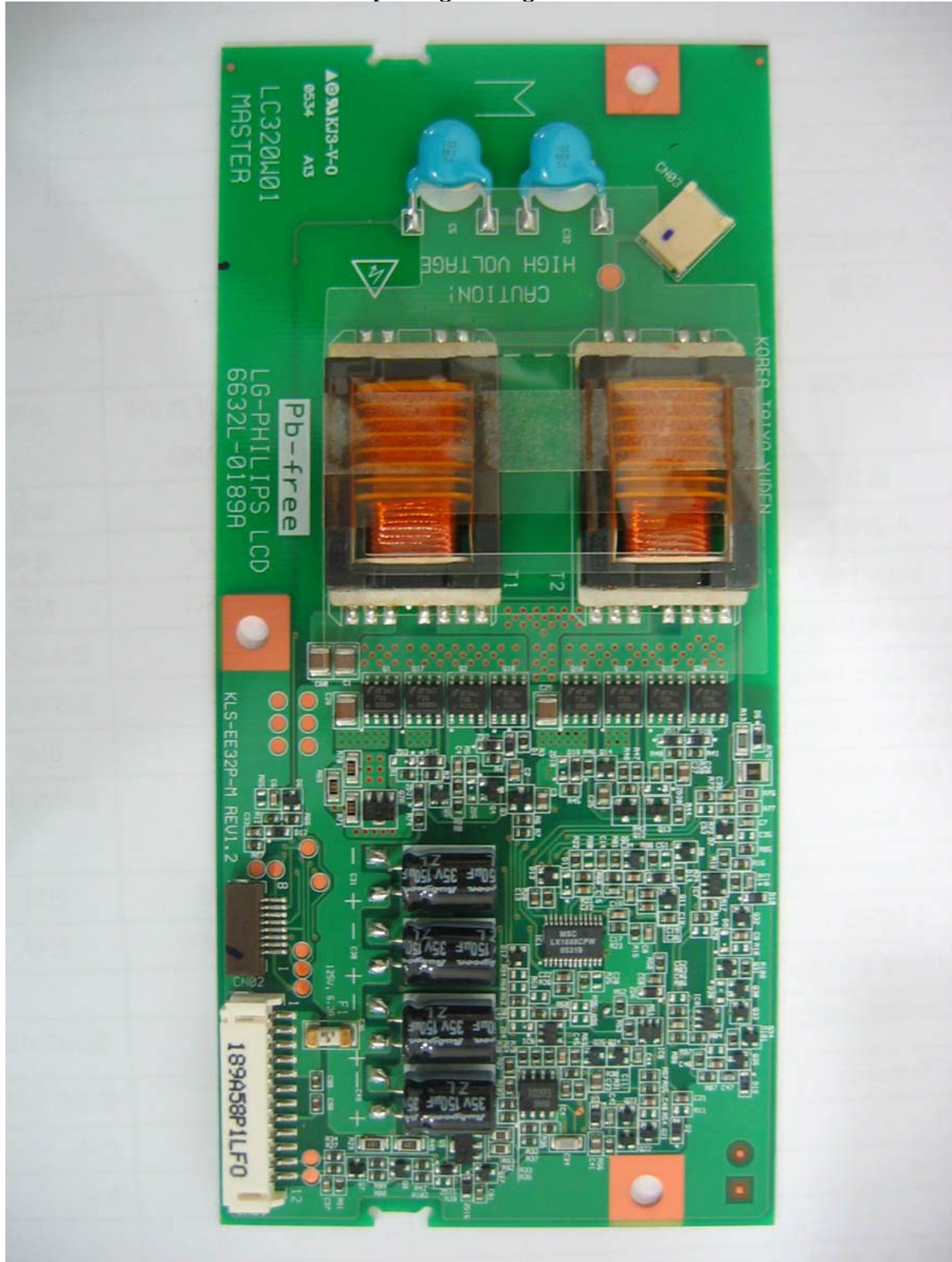
Top of high voltage board
