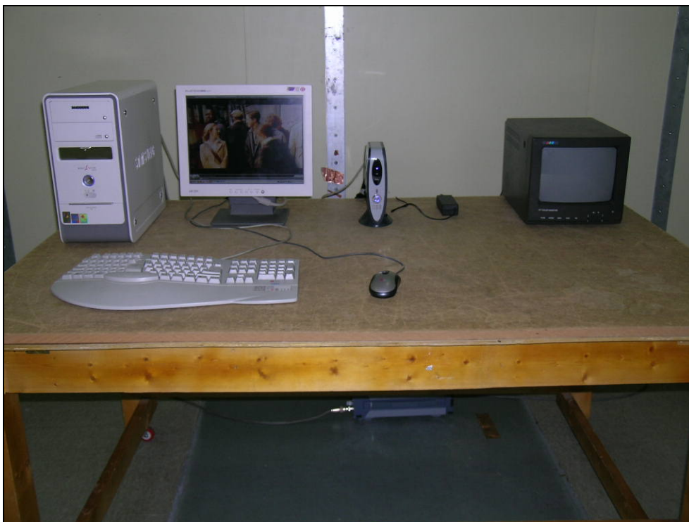
Photograph 1: Setup for Conducted Emissions
