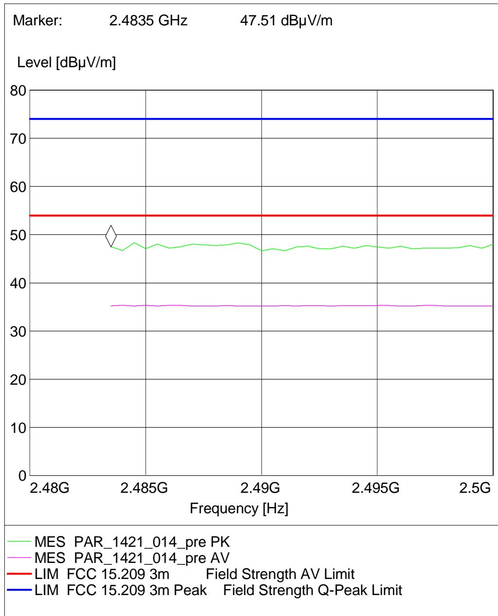
**Test: 15c.6; Frequency = 2480, Mode = BT transmit using 3 Mbps with 8DPSK modulation, Method = radiated**
