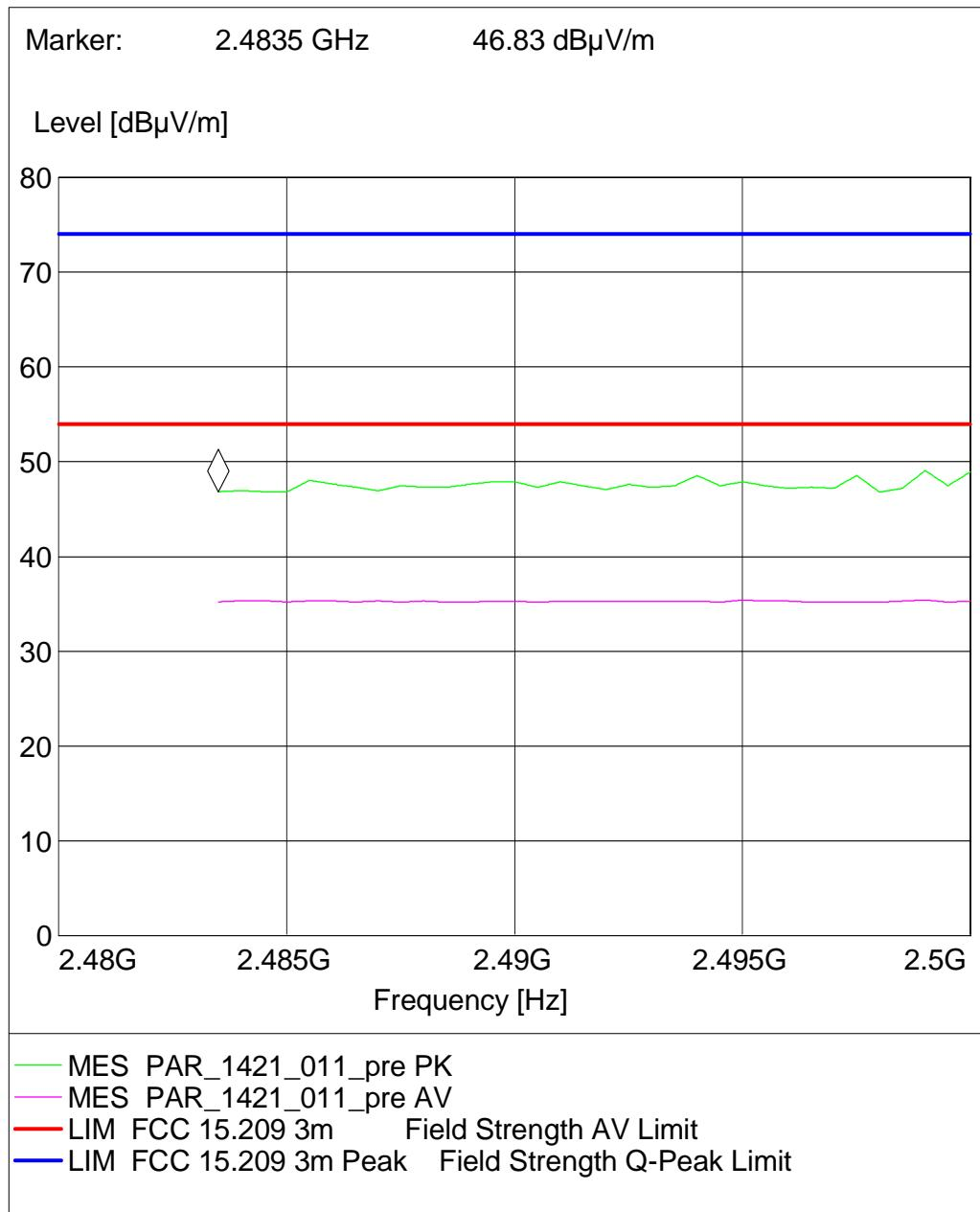
**Test: 15c.6; Frequency = 2480, Mode = BT transmit using 2 Mbps with PI/4 DQPSK modulation,
