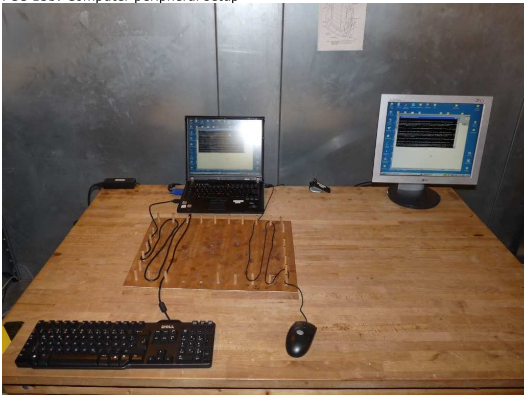
Photo 2: Test setup for conducted measurements, AC Mains FCC 15b: Computer peripheral setup
