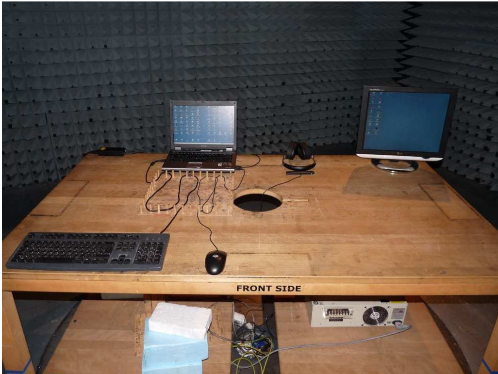
Photo 1: Test setup for radiated measurements (30 MHz to 1 GHz), FCC 15b: Computer peripheral setup
