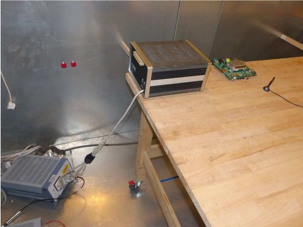
Photo 5: Test setup for conducted measurements (unintentional radiator §15)
