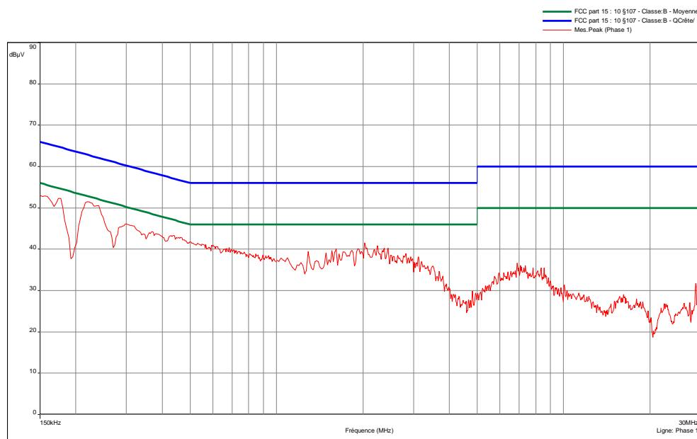
The frequencies which are not 6 dB under the Average limit are then analyzed with Average detector.
