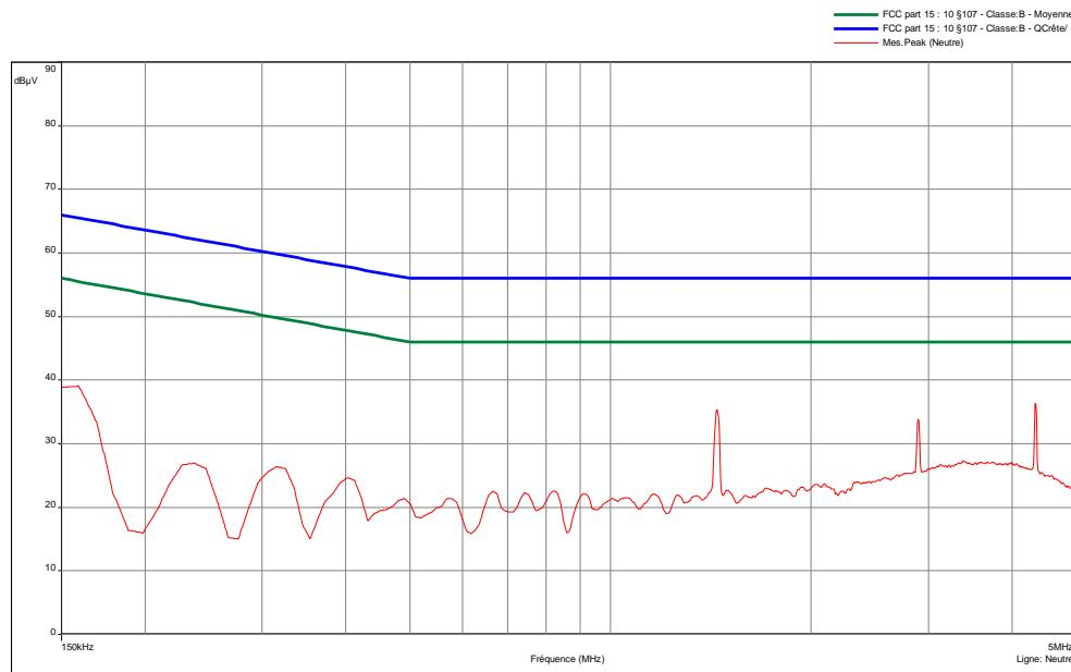
Curve N° 4: average measurement on the Line, for the frequency range: 150 kHz – 5 MHz
