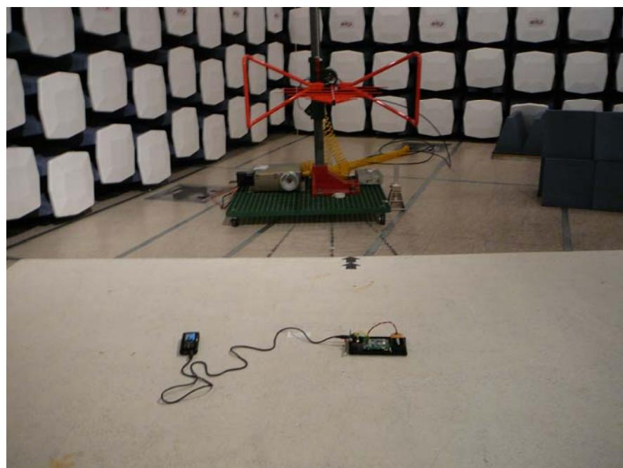
**13.7 Radiated Emission above 1 GHz (EUT with Integral Antenna) – Front View**
