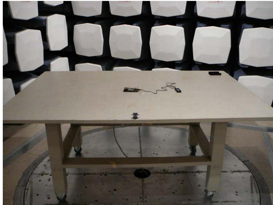
**13.8 Radiated Emission above 1 GHz (EUT with Integral Antenna) – Rear View**
