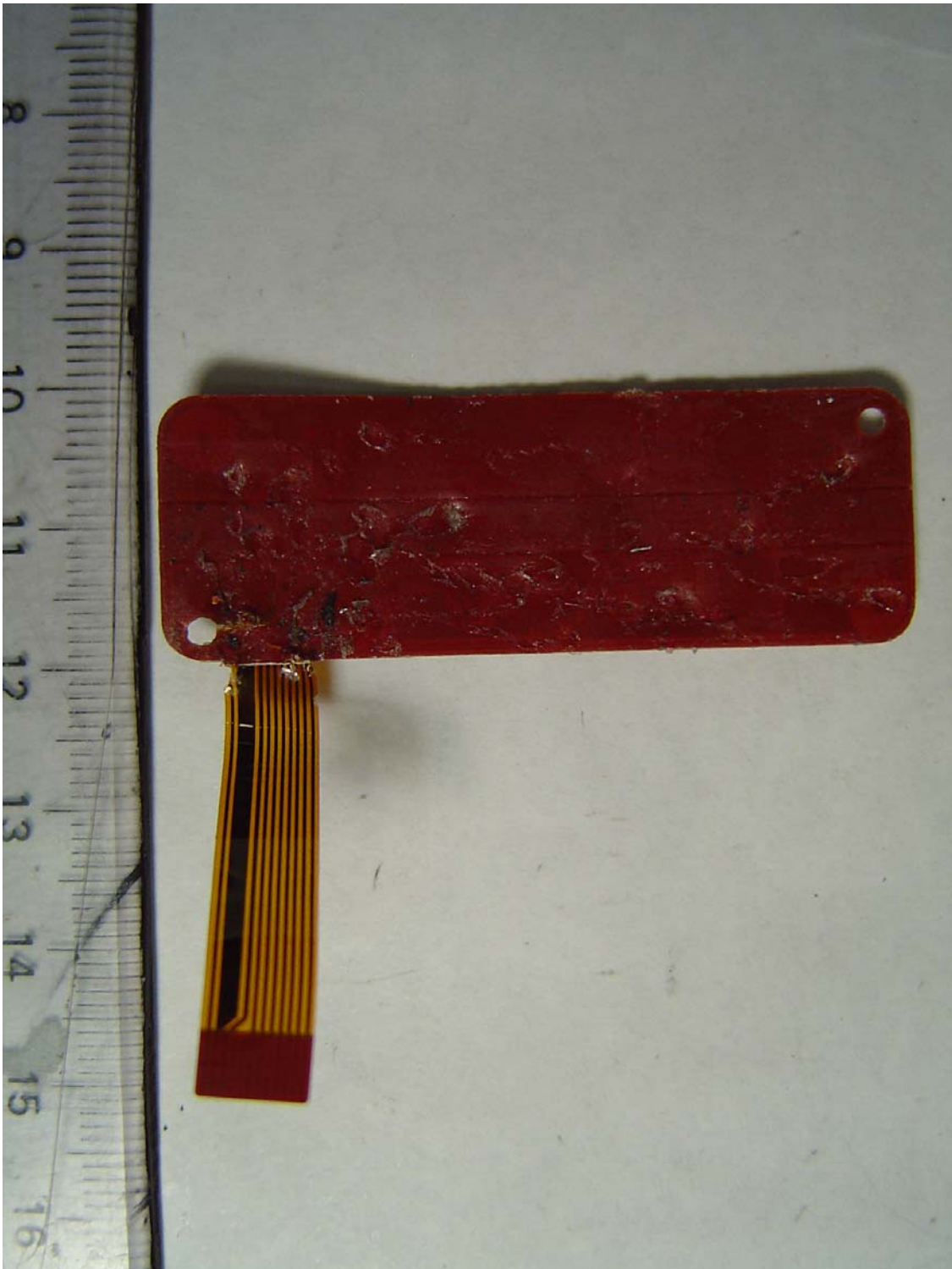
EUT Keypad Flexible Circuit – Rear View
