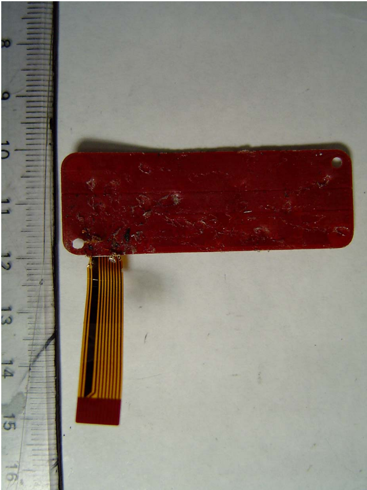
EUT Keypad Flexible Circuit – Rear View
