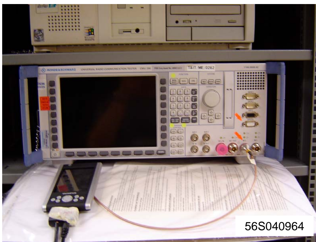
Maximum Peak Power Measurement Test Setup
