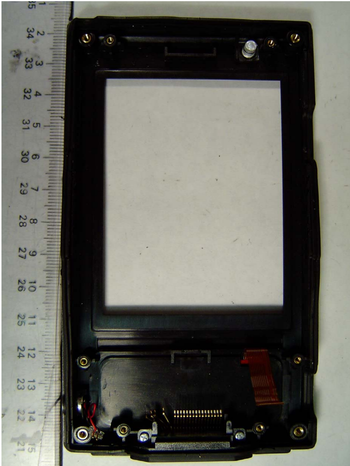
EUT Front Housing Internal View (With Display Removed)
