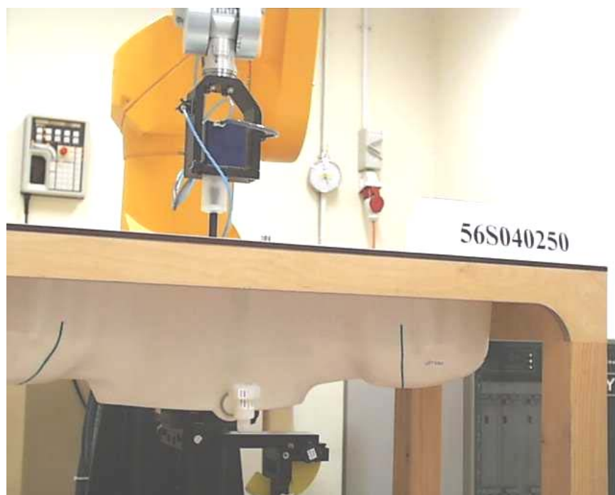
SAR Test Setup (Device at Flat Phantom)
