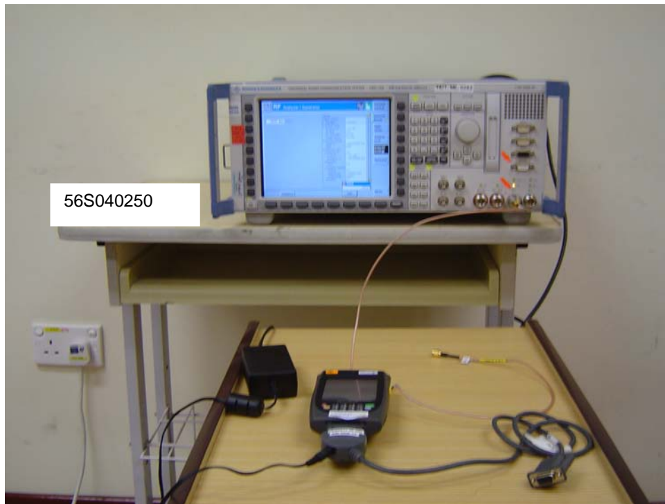
Maximum Peak Power Measurement Test Setup
