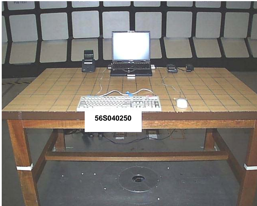
Radiated Emissions Setup (Front View)
