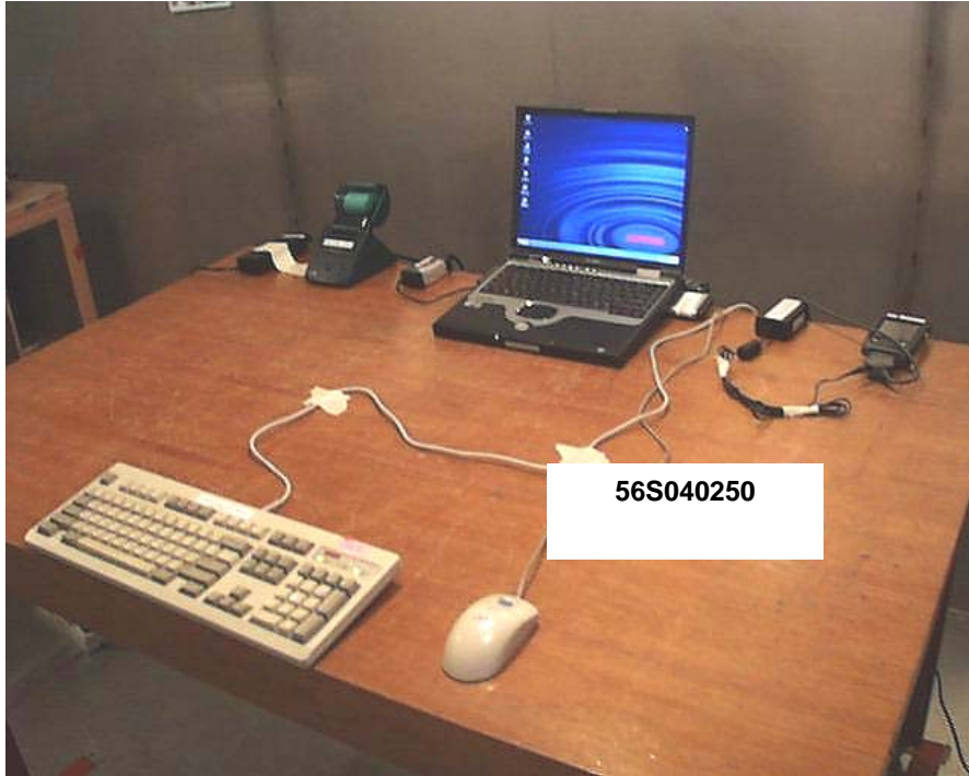
Conducted Emissions Setup (Front View)
