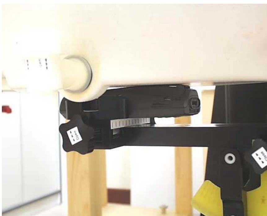
SAR Test Setup At Flat Phantom – Closer View (EUT Rear Touched Phantom)
