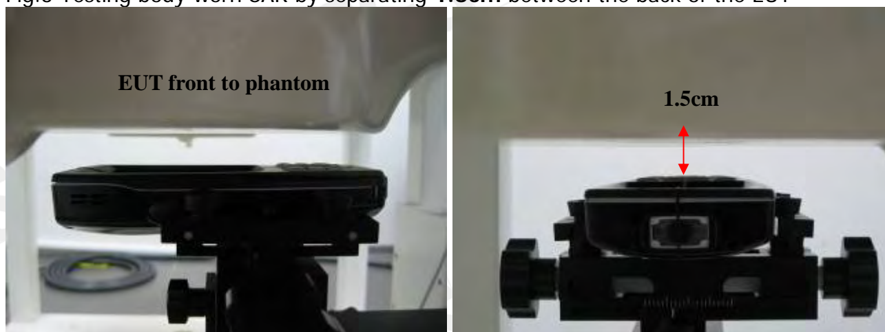
Fig.4 Testing body-worn SAR by separating 1.5cm between the front of the EUT
