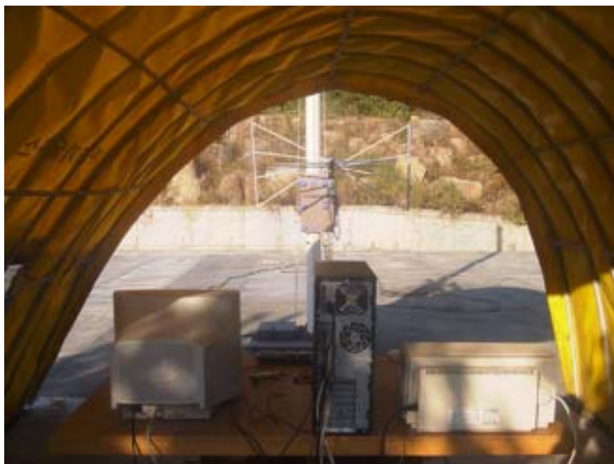
Photograph 1 : Setup for radiated Emissions
