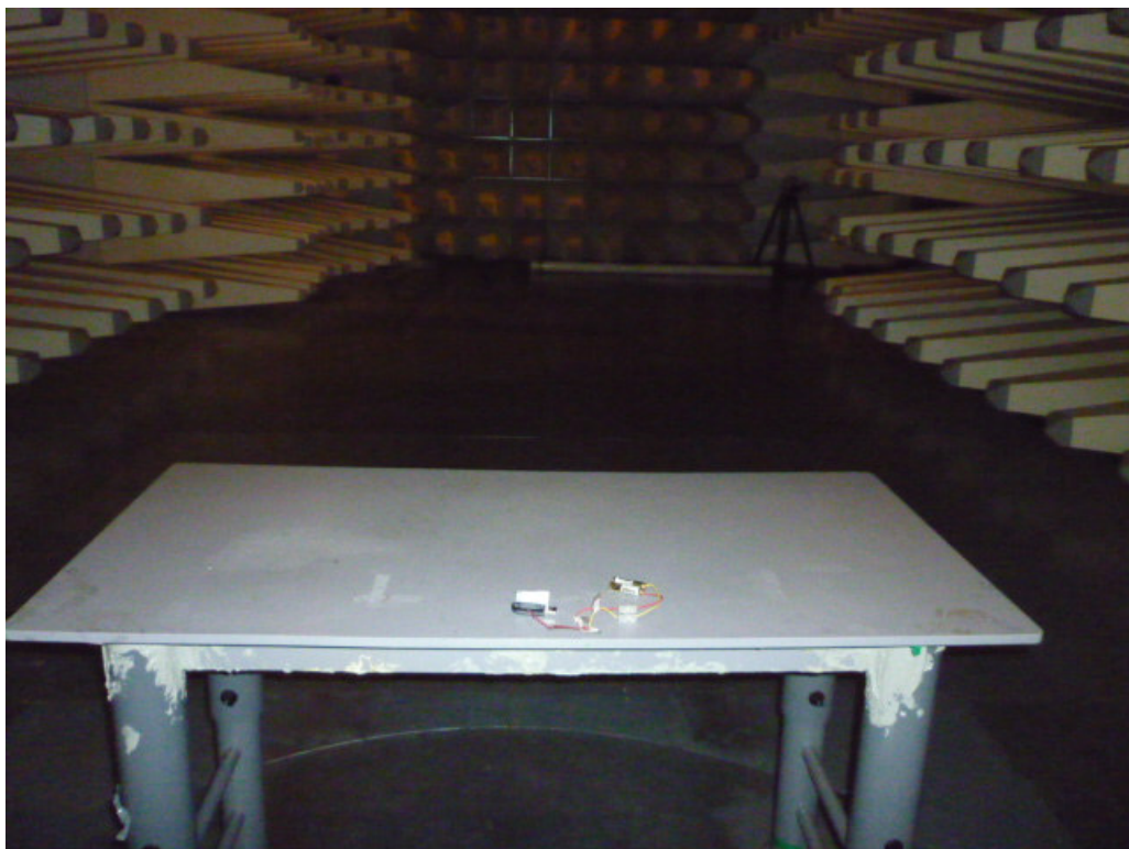
Set-up for Radiation Emission (Transceiver)
