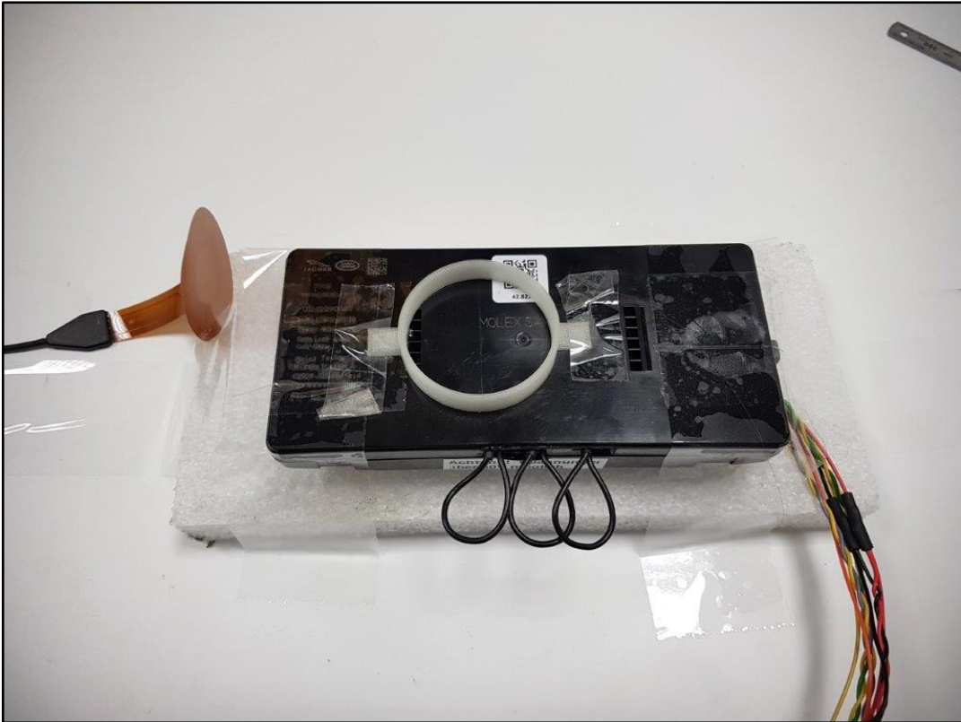
Photo 5: Test pictures - Setting probe to the centre of the coil 3
