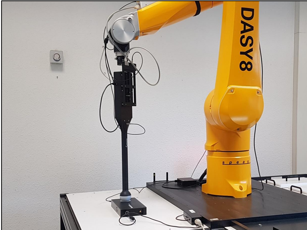
Photo 1: DASY 8 WPT set up
